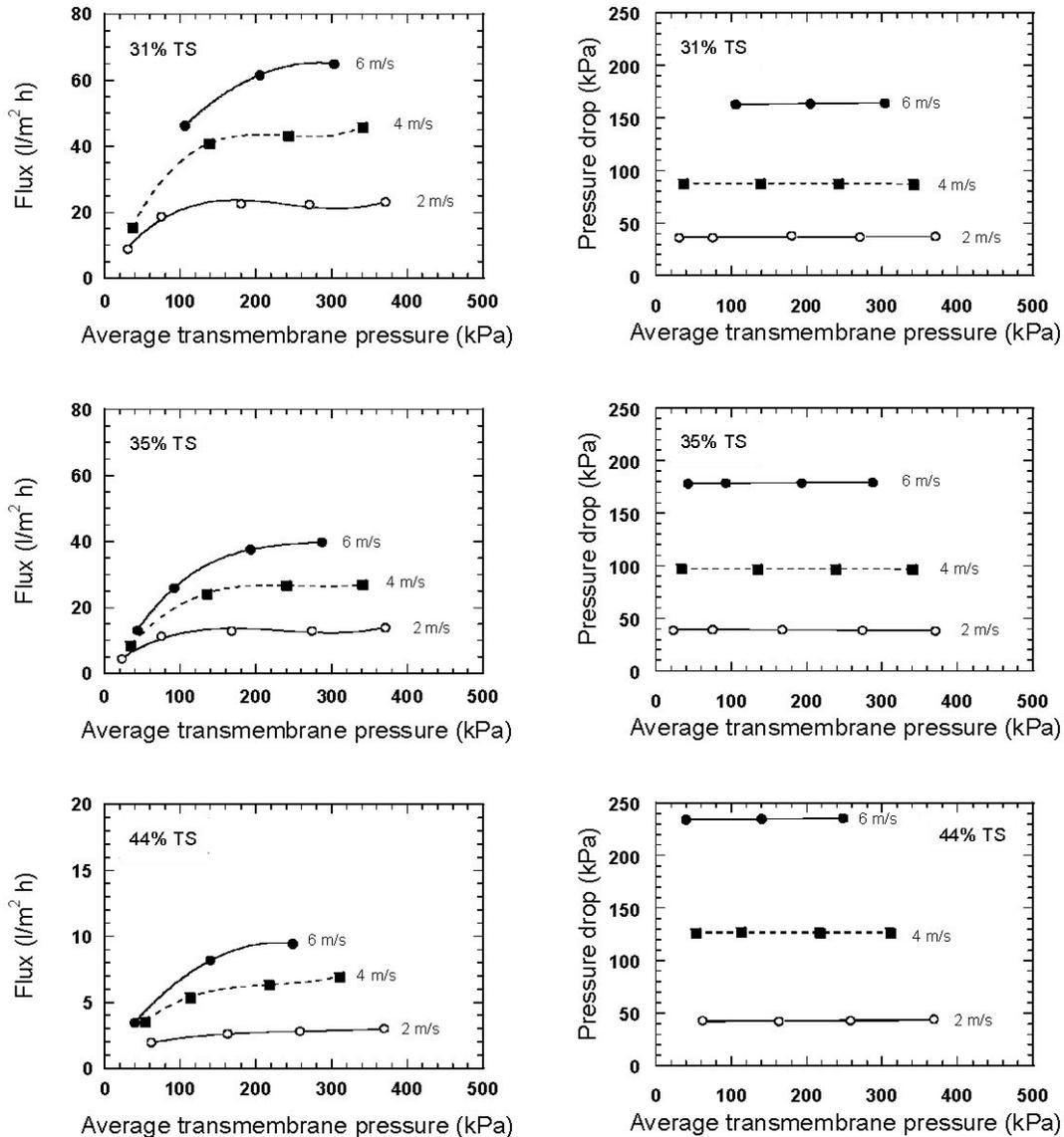
Fig. 2. Influence of TMP and cross-flow velocity on flux (left) and frictional pressure drop (right) during ultrafiltration of hardwood black liquor with three different TS contents. Temperature was 90°C during all experiments. Symbols represent experimental data and lines second and third-degree polynomial (flux) and linear (pressure drop) fits to experimental data.
