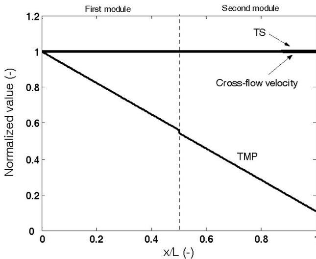
Fig. 4. Predicted TS content, cross-flow velocity and transmembrane pressure, along the flow channel at 90°C. Values are normalized to the values at the inlet of the module: TMP, 200 kPa; cross-flow velocity, 4 m/s; TS, 31%.
