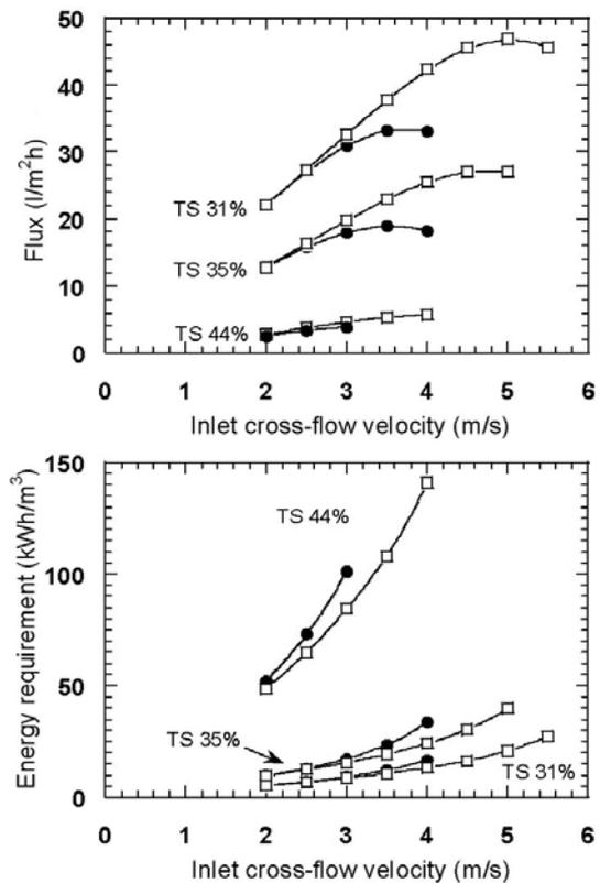
Fig. 9. Calculated average flux (above) and energy requirement (below) at three feed concentrations. Pump efficiency was set to 0.8. □: inlet TMP, 300 kPa; and ●: inlet TMP, 200 kPa.
