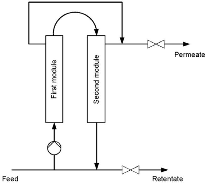
Fig. 3. Unit with two membrane modules in series.
