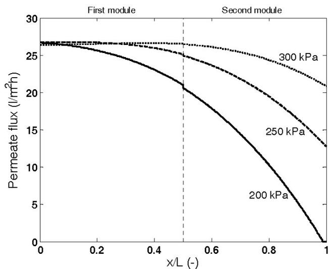
Fig. 8. Flux along the flow channel for evaporated black liquor with a ceramic membrane at different TMPs at the inlet of the first module. Cross-flow velocity at the inlet, 4 m/s; TS of feed solution, 35%.
