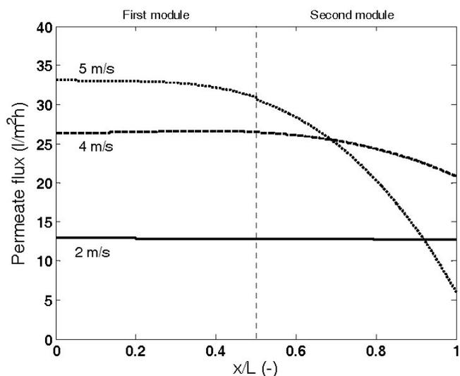
Fig. 7. Flux along the flow channel at various inlet cross-flow velocities. TMP at the inlet, 300 kPa; TS of feed solution, 35%.
