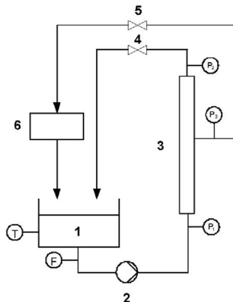
Fig. 1. Schematic illustration of the equipment used in the UF experiments. 1 feed tank, 2 pump, 3 membrane module, 4 retentate valve, 5 permeate valve, 6 balance. T: temperature regulator, F: flow meter,  $P_1$ ,  $P_2$ ,  $P_3$ : pressure transmitters.
