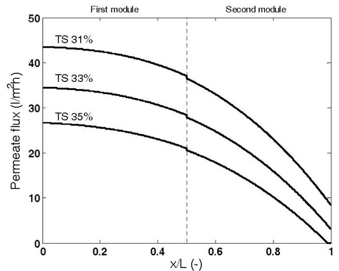
Fig. 6. Predicted permeate flux along the flow channel for three concentrations of black liquor at 90°C. TMP, 200 kPa; cross-flow velocity, 4 m/s.
