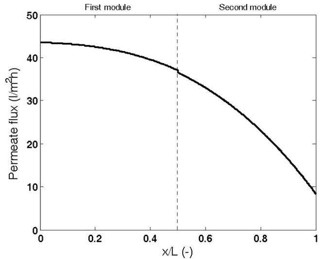
Fig. 5. Predicted permeate flux along the flow channel. Same basic data as in Fig. 4 were used for the simulations.
