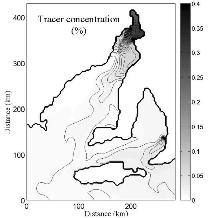
Fig. 8. Far-field study. Simulated distribution of concentration of discharge water (%) for austral winter.
