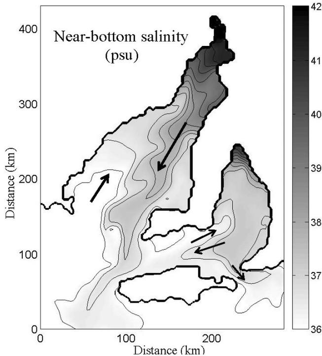
Fig. 5. Far-field study. Simulated distribution of near-bottom salinity for austral winter. Arrows indicate flow directions.
