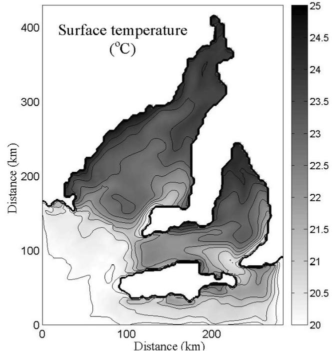
Fig. 6. Far-field study. Simulated distribution of surface temperature (°C) for austral summer.
