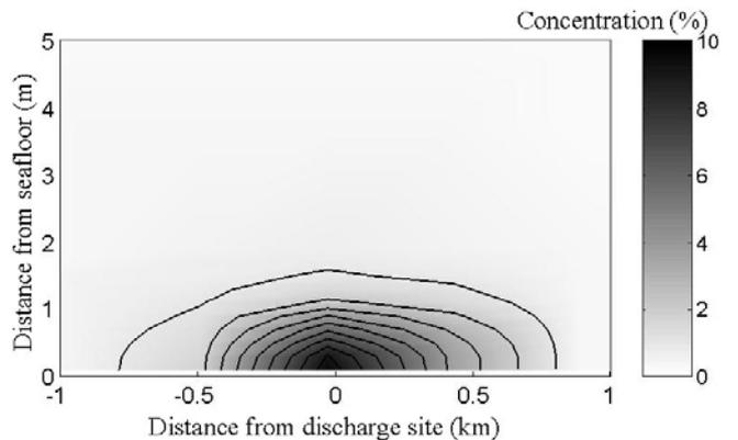
Fig. 10. Snapshot of the concentration of discharge water (%) in vicinity of the Spencer Gulf discharge site.
