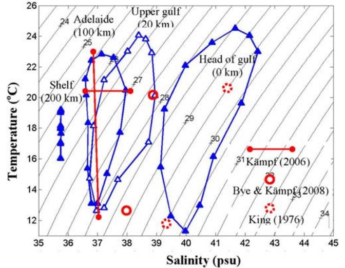
Fig. 4. Far-field study. Simulated monthly mean (triangles) and observed (circles) values of temperature and salinity at selected locations in Gulf St. Vincent. Lines indicate observed ranges. Contour lines refer to true density minus 1000 kg/m<sup>3</sup>. Distances are given with respect to the head of gulf.
