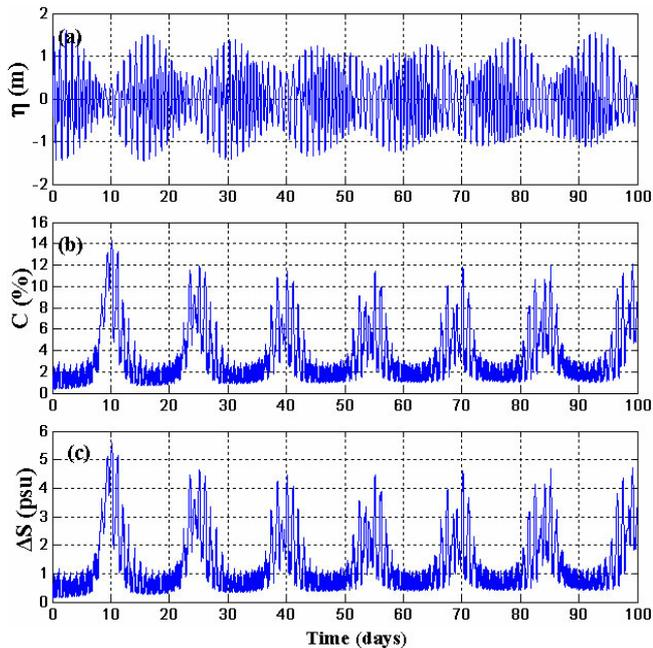
Fig. 11. Near-field study. Evolutions of (a) sea level (m), (b) concentration of discharge water (%), and (c) salinity excess at the Spencer Gulf discharge site.
