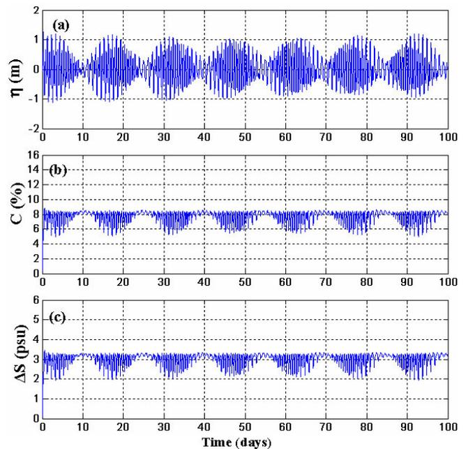
Fig. 12. Near-field study. Evolutions of (a) sea level (m), (b) concentration of discharge water (%), and (c) salinity excess at the Gulf St. Vincent discharge site.
