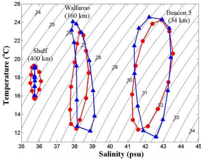
Fig. 3. Far-field study. Simulated monthly mean (triangles) and observed (full circles) values of temperature and salinity at selected locations in Spencer Gulf. Contour lines refer to true density minus 1000 kg/m<sup>3</sup>. Distances are given with respect to Port Augusta. Observations are taken from Nunes and Lennon [21].
