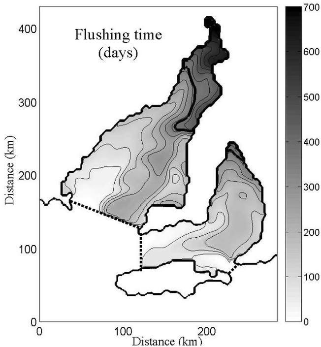
Fig. 7. Far-field study. Simulated distribution of flushing time (days) for austral winter. Thick lines highlight a flushing time of one year. Dotted lines are the assumed boundaries between gulf and shelf water used for the flushing time calculations.
