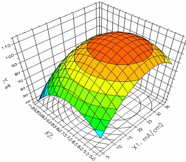
Fig. 3. 3D response surface plots for turbidity removal vs. current density and pH, MWE 5% (in wt.), pH = 7.
