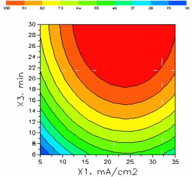
Fig. 4. Contour plots of turbidity removal vs. current density and treatment time, MWE 5% (in wt.), pH = 7.
