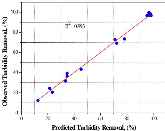
Fig. 1. Relation between experimental and predicted turbidity removal using Eq. (3).
