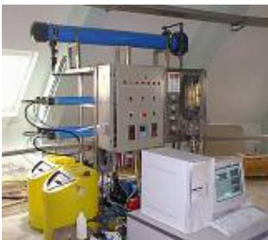
Fig. 19. SWRO desalination plant.
