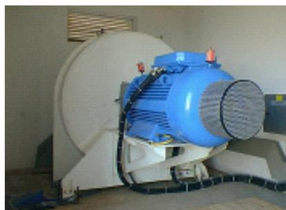
Fig. 6. 100 kVA synchronous machine coupled to flywheel.
