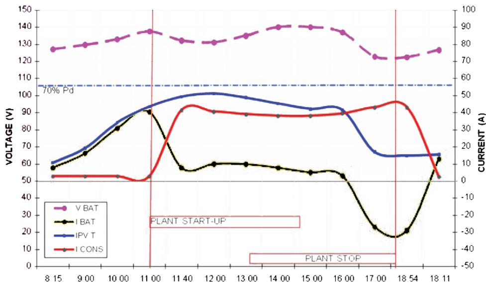
Fig. 27. Ksar Ghilène functioning system, daily energy flow.
