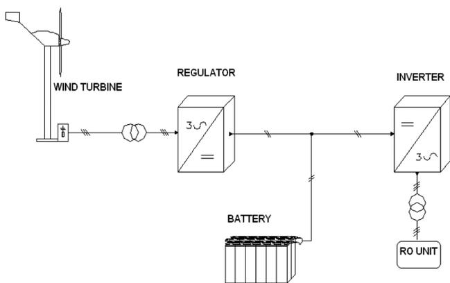
Fig. 11. System configuration of autonomous wind RO system.
