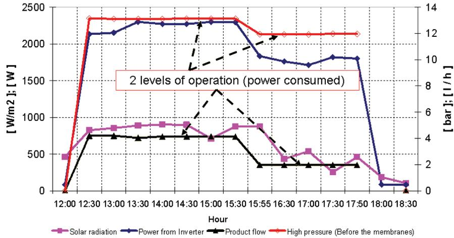
Fig. 28. Ksar Ghilène functioning system, operation case of variable power consumption.
