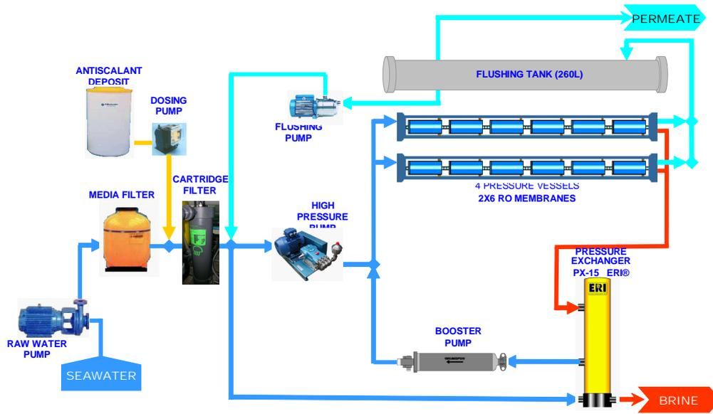
Fig. 22. SWRO desalination plant configuration.
