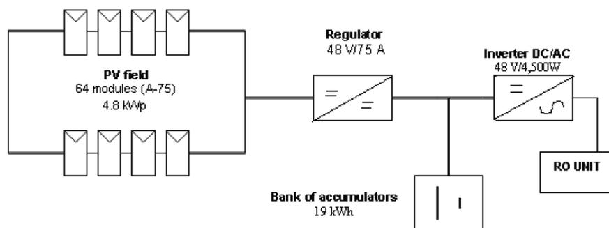
Fig. 18. Basic diagram of PV-RO concept.
