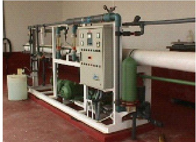
Fig. 2. SWRO desalination plant.
