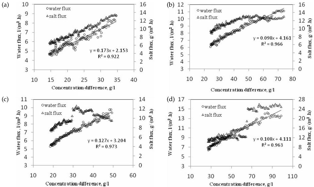
Fig. 4. Profiles of permeate water flux and salt flux at draw solution initial concentrations of (a) 35 g/l, (b) 50 g/l, (c) 75 g/l, and (d) 100 g/l against tap water as feed.
