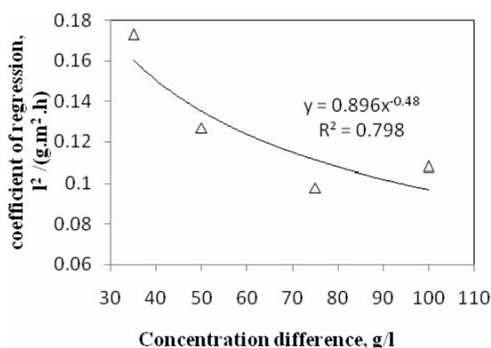
Fig. 6. Effect of initial concentration of draw solution on values of coefficients of regression.
