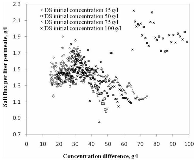
Fig. 7. Salt transported from a draw solution into feed water per liter permeated water.
