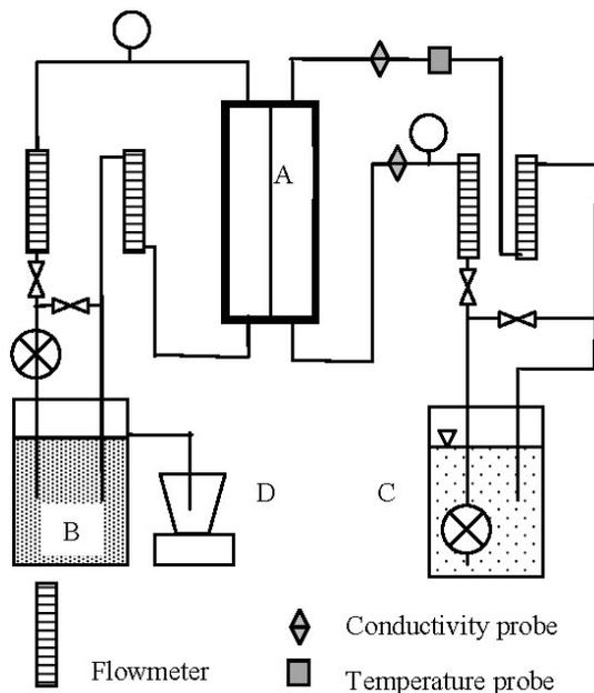
Fig. 2. Experimental set-up used for membrane module test. A, membrane module; B, osmotic solution reservoir; C, feed water reservoir; D, beaker on digital balance.
