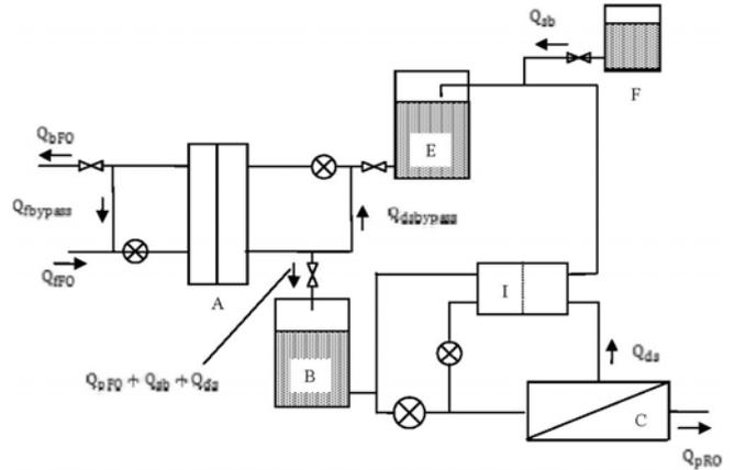
Fig. 8. Main components and design parameters of a conceptual integrated FO–RO system. A, FO module; B, FO permeate reservoir; C, RO module; D, pressure exchanger; E, RO brine reservoir; F, concentrated salt brine reservoir.
