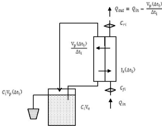
Fig. 3. Schematic representation of mass transfer between draw solution and feed water loops of the system.
