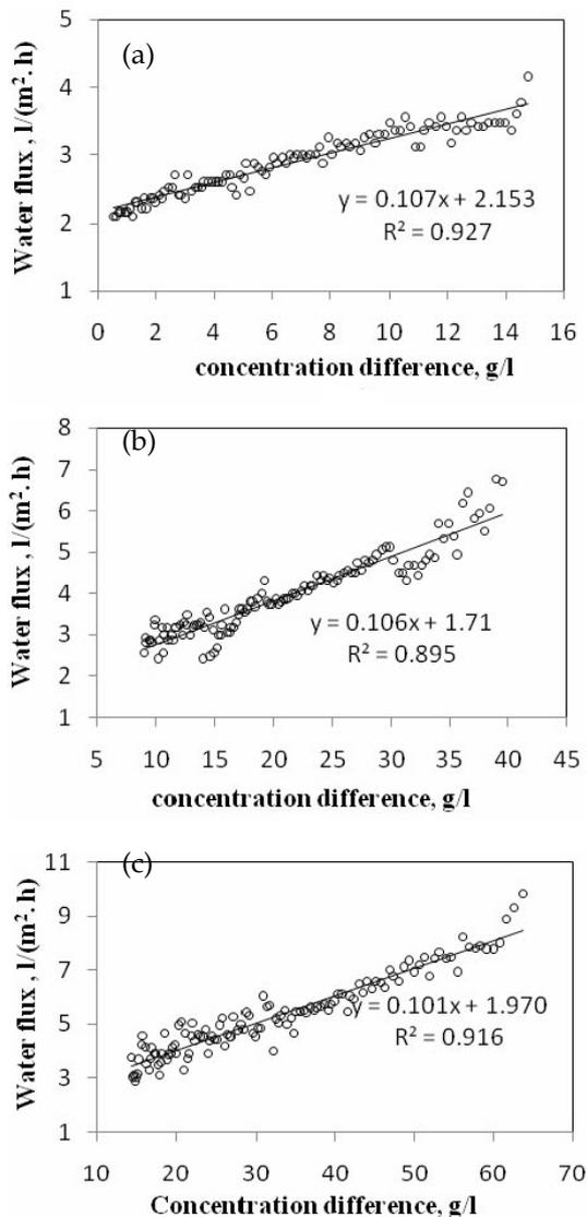
Fig. 5. Profiles of permeate water flux at draw solution initial concentrations of (a) 50 g/l, (b) 75 g/l and (c) 100 g/l against seawater as feed.
