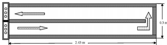
Fig. 1. Flow pattern in an unrolled HydroWell spiral-wound cartridge. Arrows show flow path of osmotic solution in the membrane envelope. Contaminated water flows tangentially across outer side of the membrane envelope [22].
