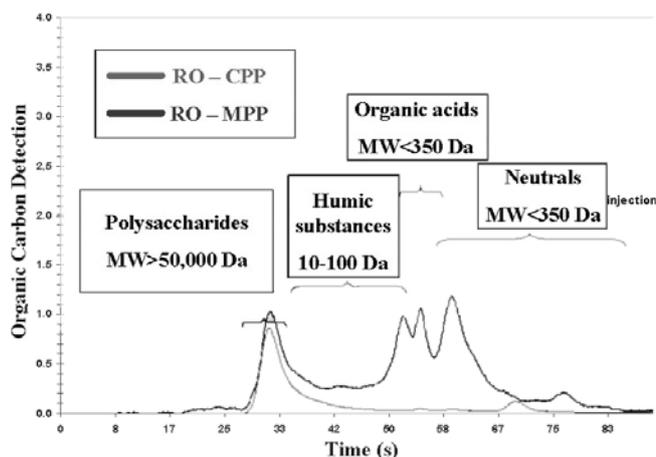
Fig. 5. LC-OCD analysis of the deposit at the surface of the RO membranes fed by CPP (in gray) and by MPP (in black).
