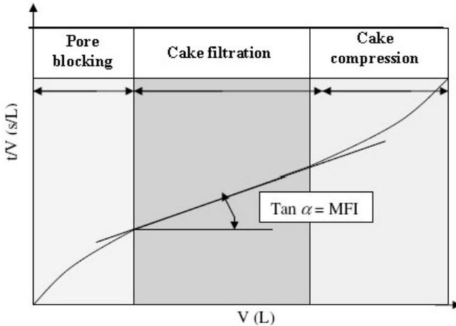
Fig. 1. Evolution of the  $t/V$  ratio as a function of  $V$ .
