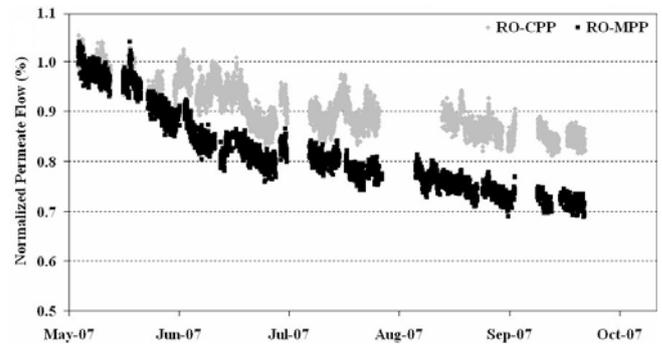
Fig. 4. Evolution of NPF/NPF<sub>0</sub> for the RO membranes fed by CPP (in grey) and MPP (in black).
