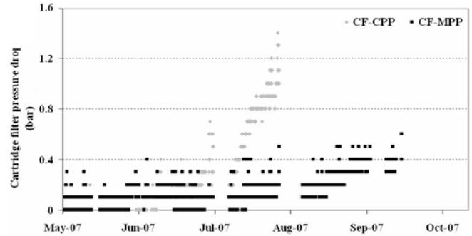
Fig. 3. Evolution of the cartridge filter pressure drop for CPP (in grey) and MPP (in black) pretreated seawater.
