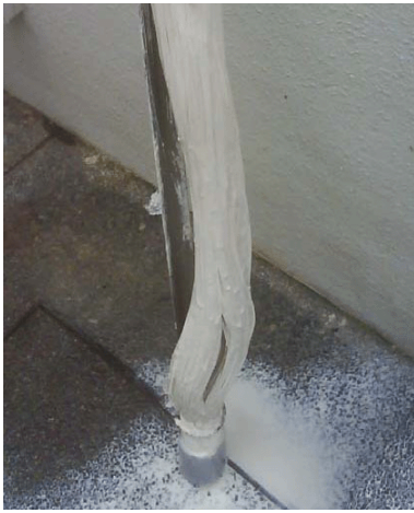
Fig. 5. Membrane coated with a thick sticky clay film after 2 and 4 Hz vibration.
