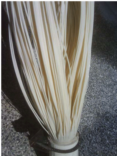
Fig. 6. Clean state of membrane with a very thin clay layer after 6 and 8 Hz vibration.
