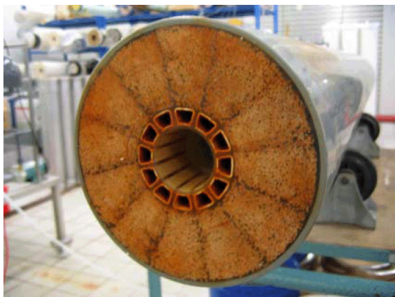
Fig. 10. UF membrane that underwent EDX analysis, confirming that red color was caused by iron with trace amounts of silica and aluminum.
