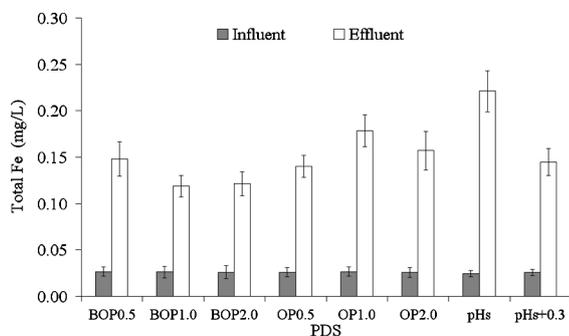
Fig. 1. Comparison of influent and effluent average iron concentration, with whiskers indicating 95% confidence interval around the mean.
