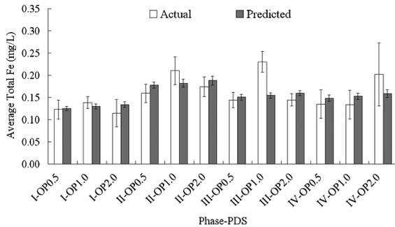
Fig. 3. Total iron release model summary for the OP PDSs by phase, with whiskers indicating 95% confidence interval around the mean.
