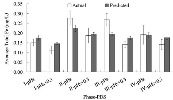
Fig. 4. Total iron release model summary for the pH control PDSs by phase, with whiskers indicating 95% confidence interval around the mean.
