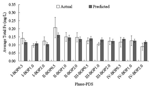
Fig. 2. Total iron release model summary for the BOP PDSs by phase, with whiskers indicating 95% confidence interval around the mean.
