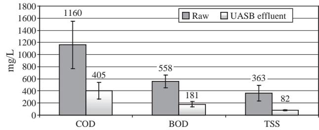
Fig. 5. Performance of UASB reactor for the treatment of blackwater.
