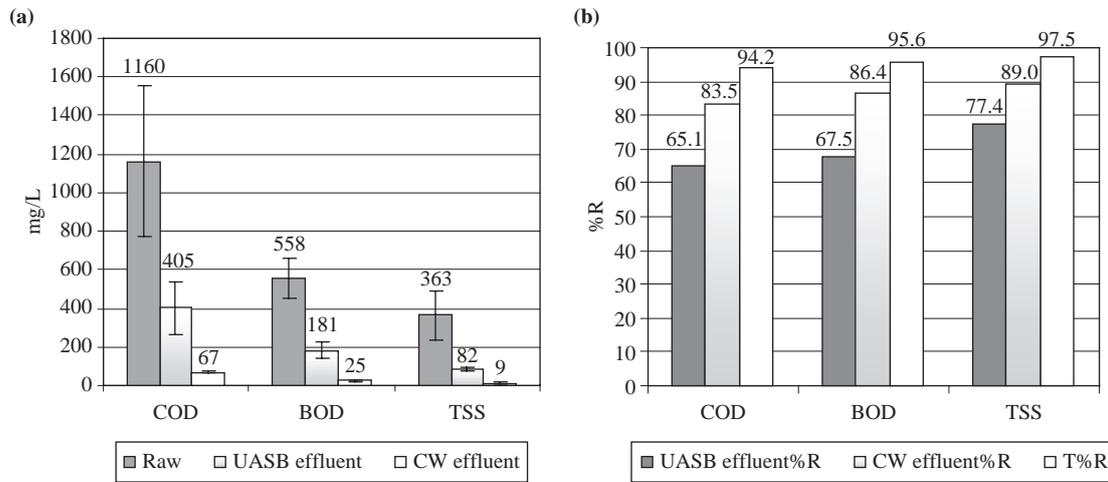
Fig. 6. Performance of the combined UASB and CW for the treatment of blackwater (a) characteristics of blackwater as well as treated effluents, (b) the corresponding percentage removal.
