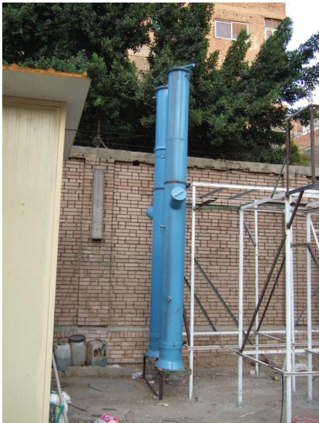
Fig. 1. UASB reactor used in the study.
