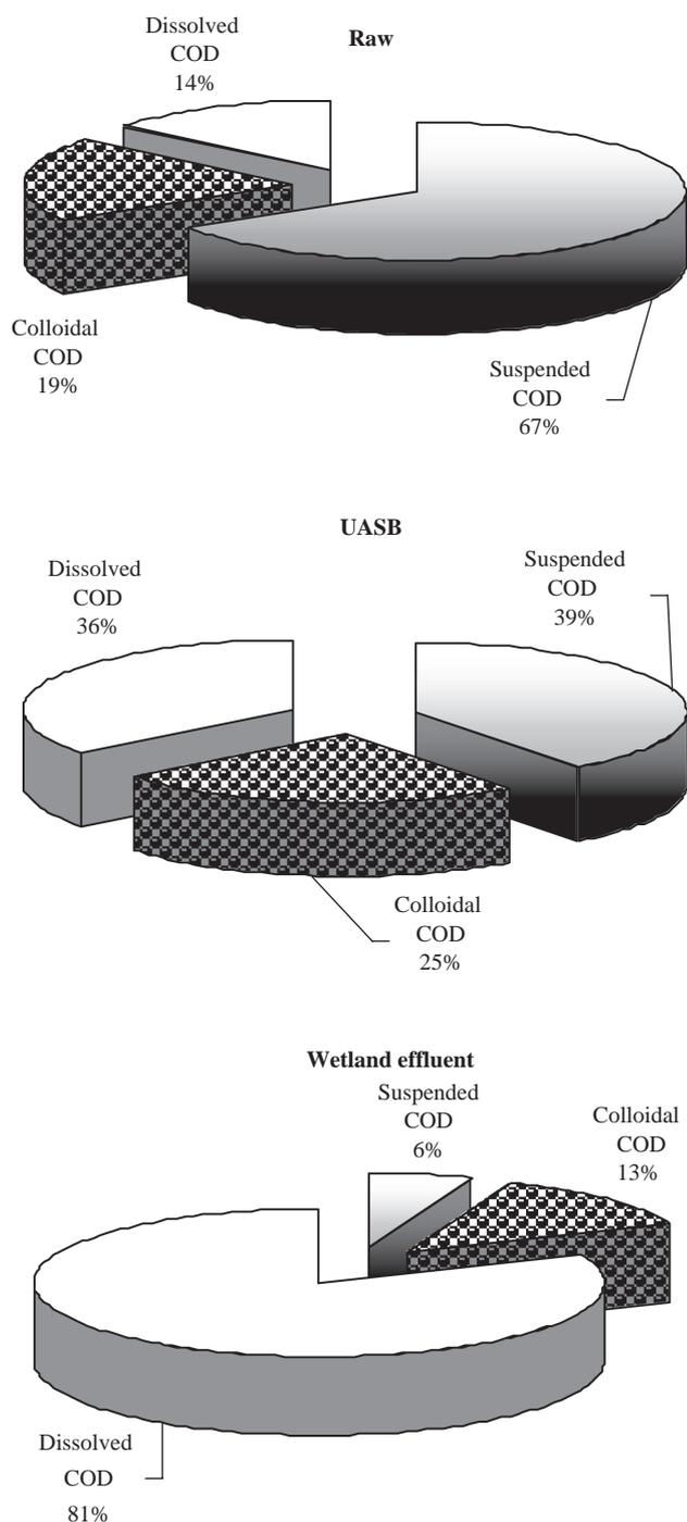
Fig. 7. COD fractions at different treatment steps for blackwater.
