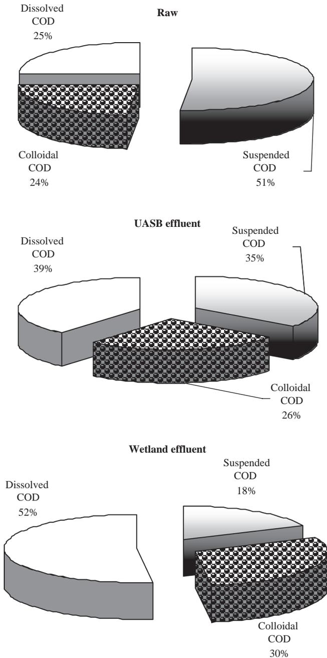
Fig. 4. COD fractions at different treatment steps for greywater.
