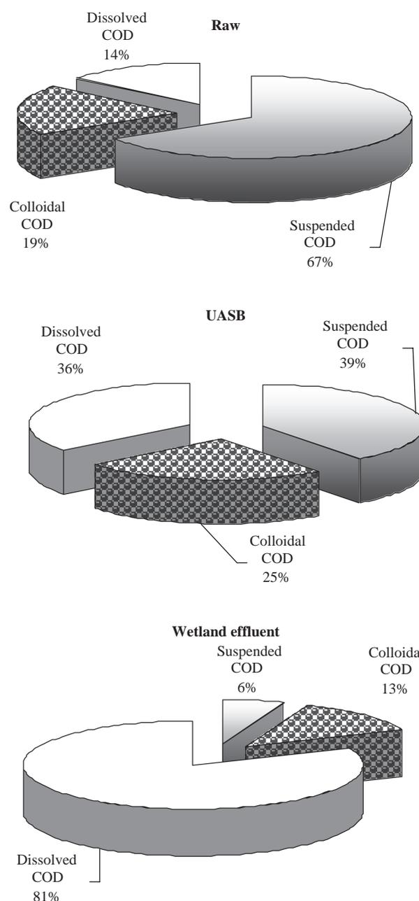
Fig. 3. COD fractions at different treatment steps for blackwater.
