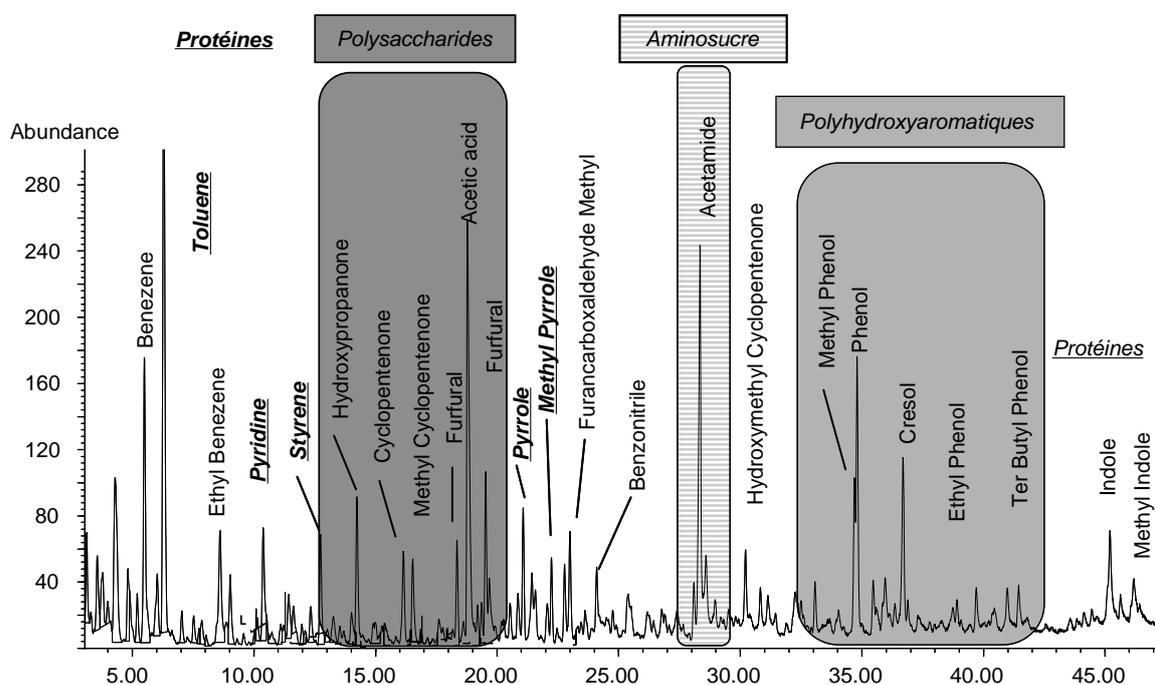
Fig. 8. Profil in pyrolysis GC/MS of the deposit of March 2008.
