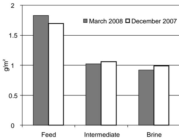
Fig. 6. Mass of dried deposit recovered on the surface of the desalination membranes.
