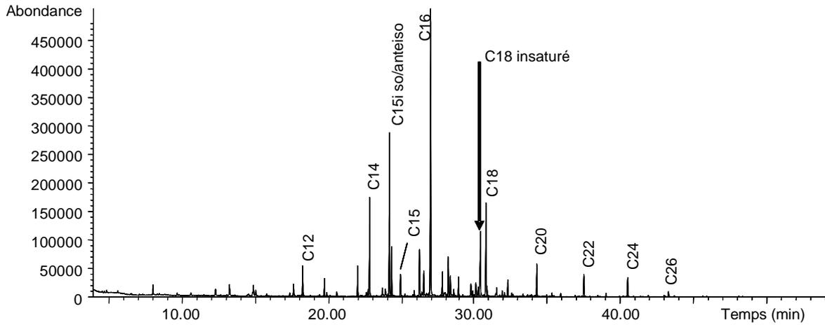
Fig. 9. Fragmentogram m/z 74 (fatty acids) in thermochemolysis GC/MS of the March 2008 deposit.
