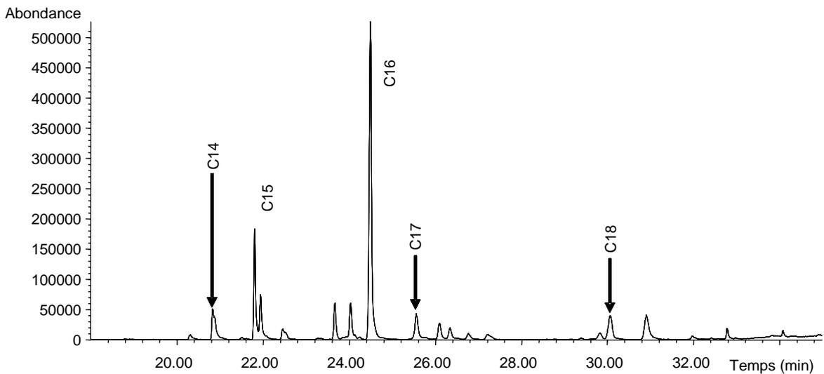
Fig. 11. Chromatogram of phospholipids analysis – March 2008 deposit.
