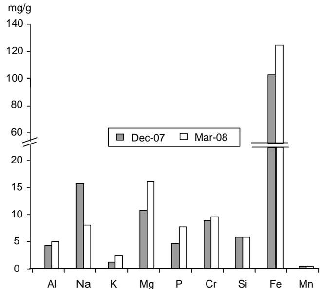
Fig. 7. ICP-OES analysis of the deposit accumulated at the surface of the desalination membranes.
