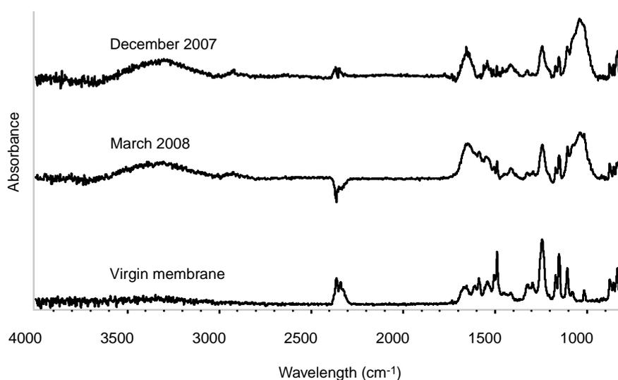
Fig. 4. Infrared spectra (FT-IR ATR) of a virgin membrane and fouled membranes of December 2007 and March 2008.
