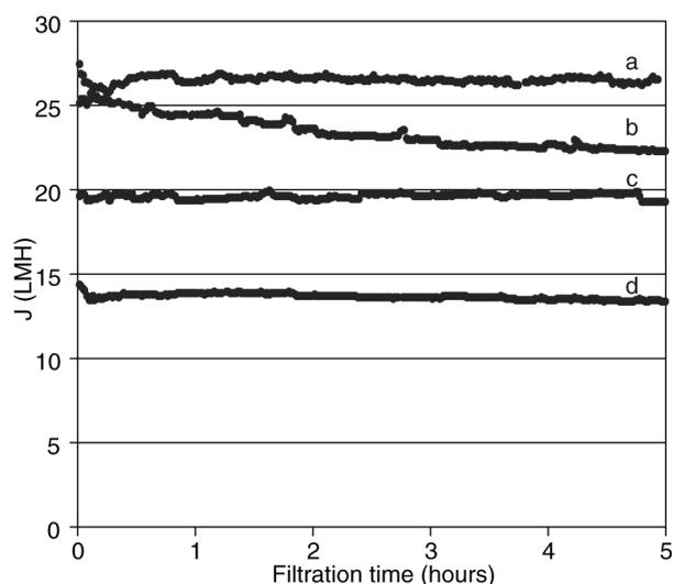
Fig. 3. Permeability tests conducted with synthetic seawater on different membranes. (a: last module/1<sup>st</sup> stage December 2007; b: membrane, manually cleaned December 2007; c and d: 1<sup>st</sup> module/1<sup>st</sup> stage March 2008 and December 2007, respectively)
