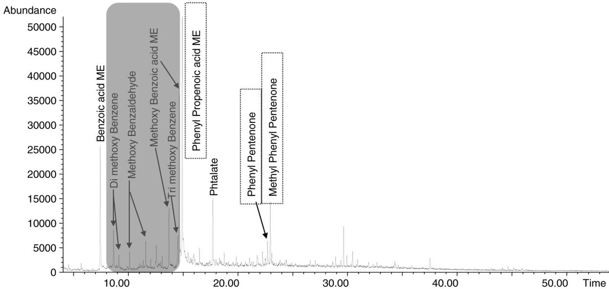
Fig. 10. Fragmentogram m/z 77 (aromatics) in thermochemolysis GC/MS of the March 2008 deposit.
