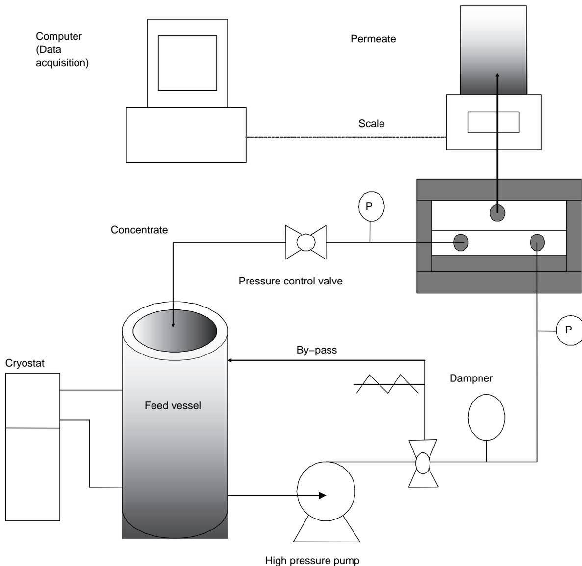
Fig. 1. Reverse osmosis unit used in the laboratory.
