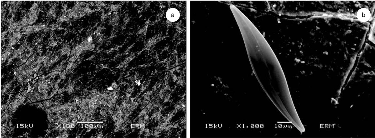
Fig. 5. SEM images of the deposit structure (a) and a diatom (b) observed on the surface of a fouled membrane of March 2008.
