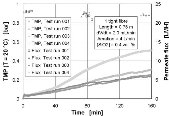
Fig. 3. Transmembrane pressure (TMP) and permeate flux vs. time for a bundle with a single, tight fibre (fibre fixed at both ends) at 4 L/min aeration rate.
