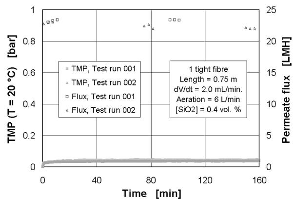
Fig. 2. Transmembrane pressure (TMP) and permeate flux vs. time for a bundle with a single, tight fibre (fibre fixed at both ends) at 6 L/min aeration rate.
