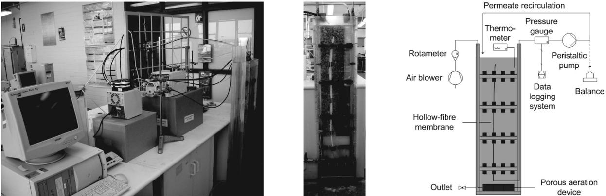
Fig. 1. Experimental setup for submerged filtration and direct observation.
