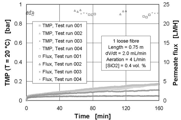
Fig. 4. Transmembrane pressure (TMP) and permeate flux vs. time for a bundle with a single, loose fibre (fibre fixed at the bottom end only) at 4 L/min aeration rate.
