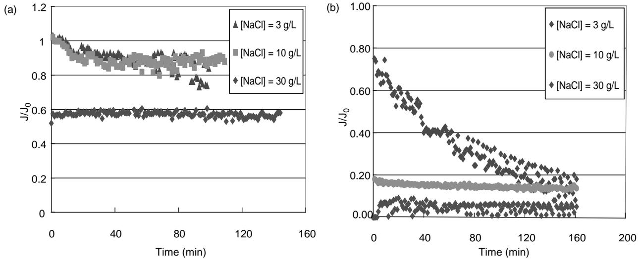
Fig. 4. Effect of concentration NaCl on the NaCl retention versus time: (a) Sepa DK, (b) NF90,  $\Delta P = 6$  bars,  $T = 25^\circ\text{C}$ ,  $\text{pH} = 6$ .
