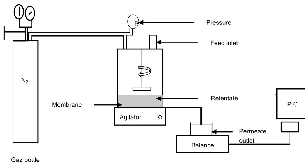
Fig. 1. Schematic diagram of nanofiltration set-up.
