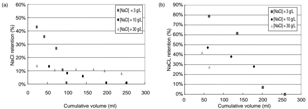
Fig. 5. Effect of concentration NaCl on the NaCl retention versus cumulative volume: (a) Sepa DK, (b) NF90,  $\Delta P = 6$  bars,  $T = 25^\circ\text{C}$ ,  $\text{pH} = 6$ .
