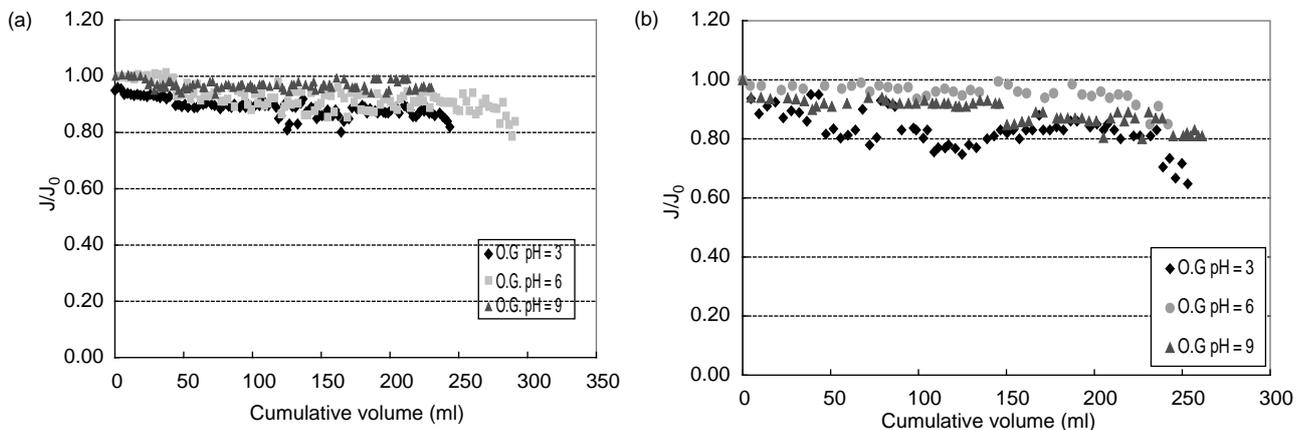
Fig. 3. Effect of pH on the relative flux ( $J/J_0$ ) versus cumulative volume: (a) Sepa DK, (b) NF90 ([O.G.] = 100 mg/L,  $\Delta P$  = 6 bars, T = 25°C).
