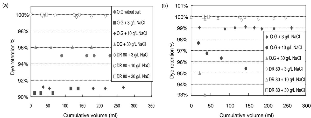
Fig. 6. Effect of NaCl concentration on the dye retention versus cumulative volume: (a) Sepa DK, (b) NF90,  $\Delta P = 6$  bars,  $T = 25^\circ\text{C}$ ,  $\text{pH} = 6$ .
