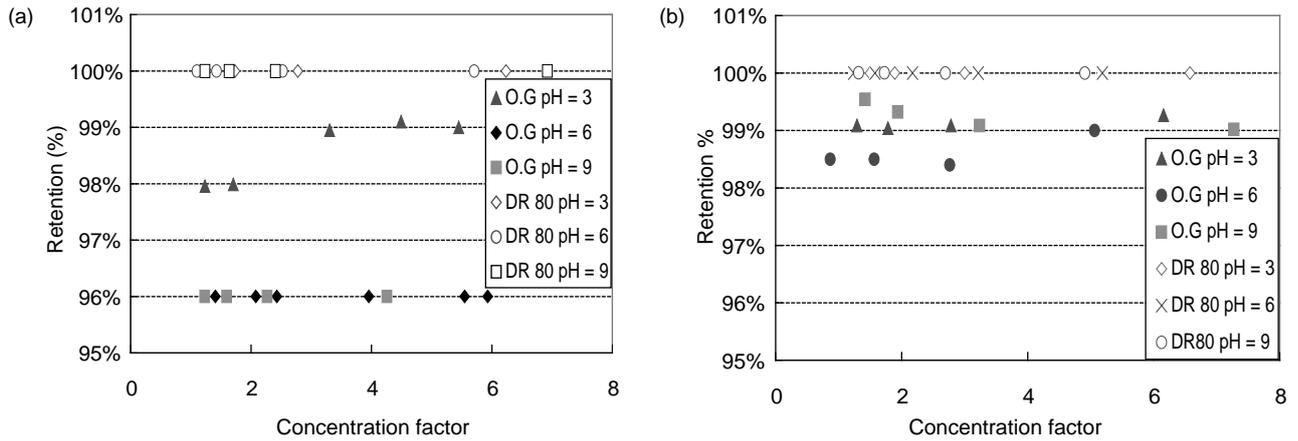
Fig. 2. Effect of pH on the dye retention versus concentration factor: (a) Sepa DK, (b) NF90, ([dye] = 100 mg/L,  $\Delta P$  = 6 bars, T = 25°C).
