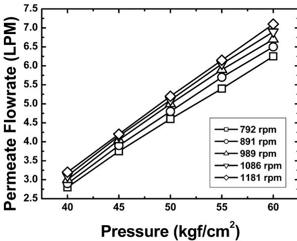
Fig. 7. Effect of rotational speed of motor and operating pressure on permeate flow rate (at 20°C).
