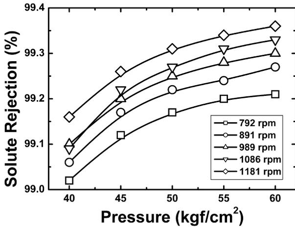
Fig. 11. Effect of rotational speed of motor and operating pressure on solute rejection (at 20°C).
