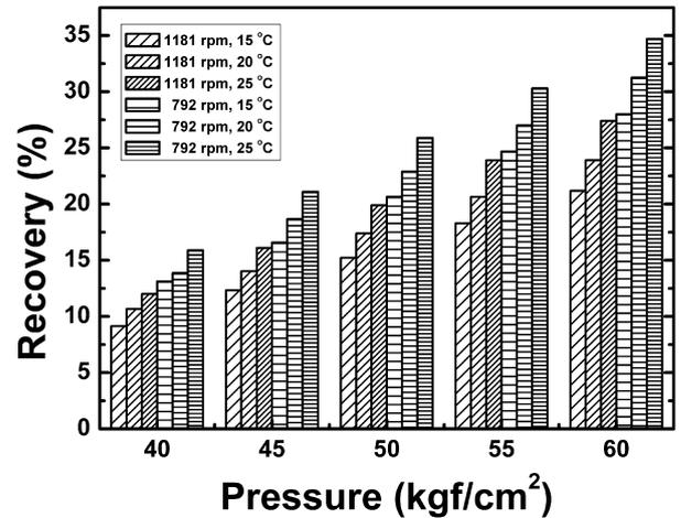
Fig. 10. Effect of feed temperature, rotational speed of motor and operating pressure on recovery ratio.
