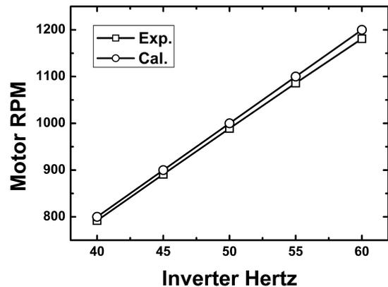
Fig. 2. Rotational speed of electric motor according to the frequency of the AC supply.
