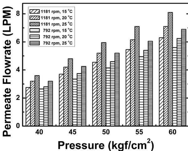
Fig. 8. Effect of feed temperature, rotational speed of motor and operating pressure on permeate flow rate.
