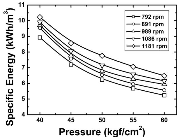
Fig. 5. Effect of rotational speed of motor and operating pressure on specific energy consumption (at 20°C).
