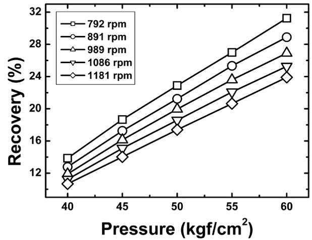
Fig. 9. Effect of rotational speed of motor and operating pressure on recovery ratio (at 20°C).
