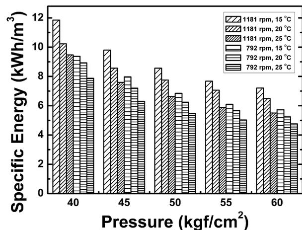
Fig. 6. Effect of feed temperature, rotational speed of motor and operating pressure on specific energy consumption.
