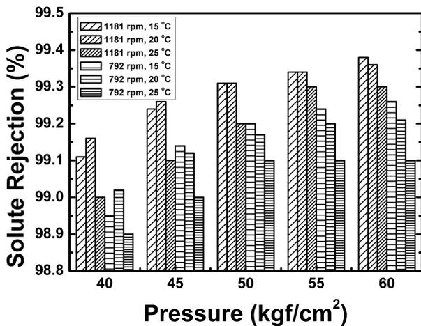
Fig. 12. Effect of feed temperature, rotational speed of motor and operating pressure on solute rejection.
