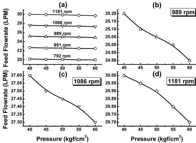
Fig. 3. Effect of rotational speed of motor and operating pressure on feed flow rate (at 20°C).
