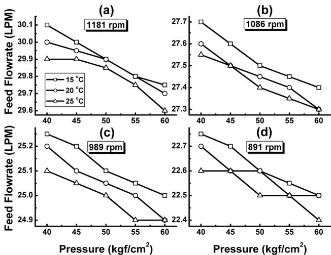
Fig. 4. Effect of feed temperature and operating pressure on feed flow rate.
