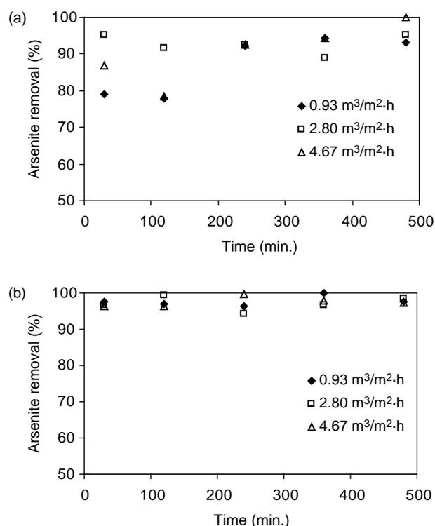
Fig. 5. Arsenite removal with the height of the filter media 45 cm (a) 0.1 mg/L and (b) 0.5 mg/L initial arsenite concentrations.
