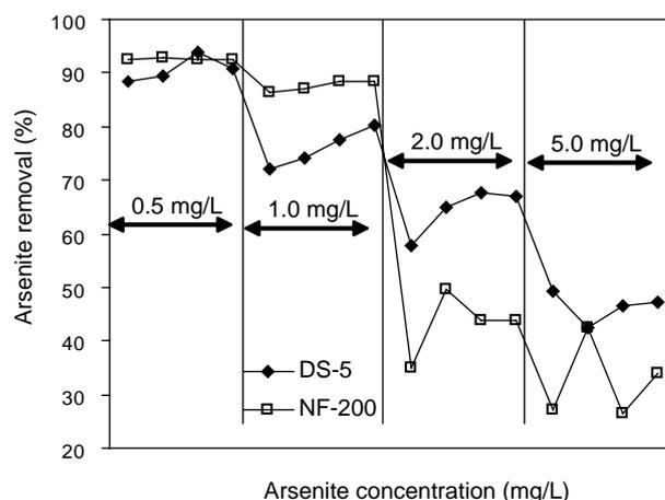
Fig. 3. Influence of the arsenite concentration on the arsenite removal by NF200 and DS5 nanofiltration membranes.
