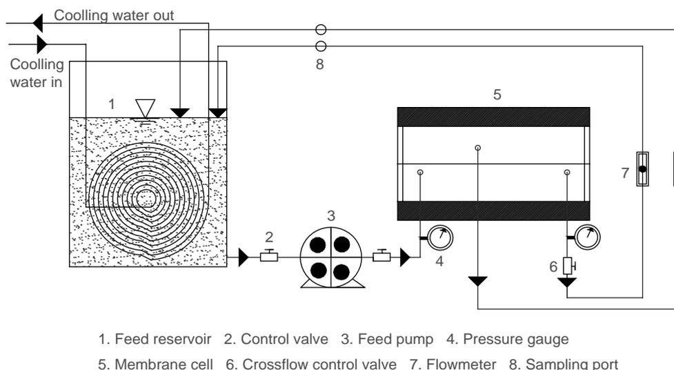
Fig. 1. Schematic diagram of laboratory scale membrane unit.
