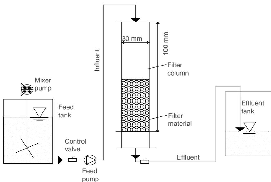
Fig. 2. Schematic diagram of laboratory scale filter column unit.
