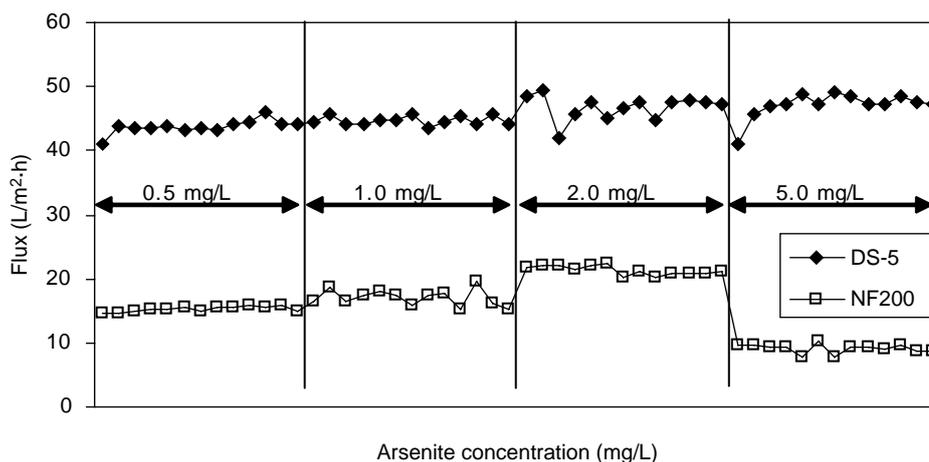
Fig. 4. Influence of the arsenite concentration on permeate flux.
