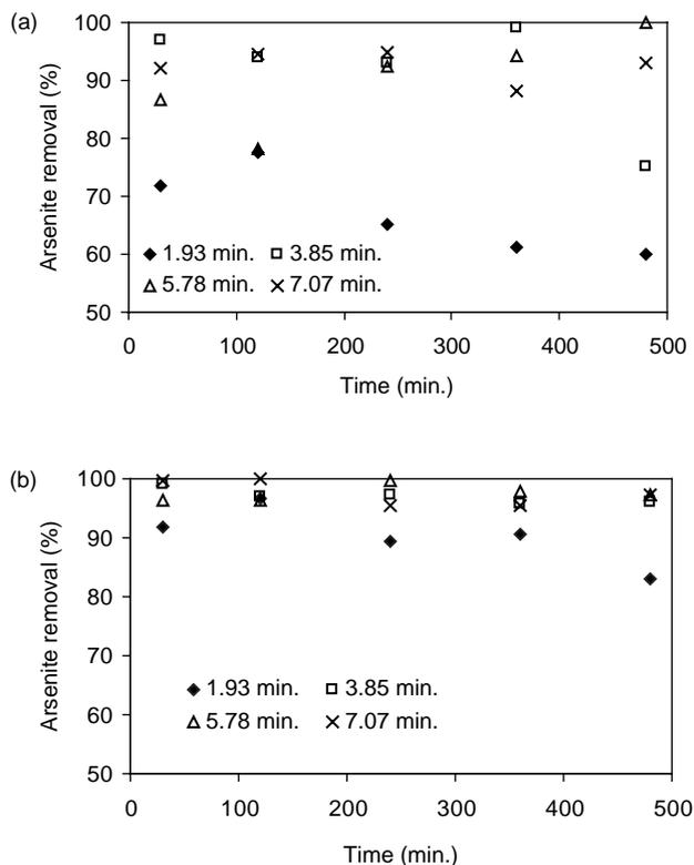
Fig. 6. Contact time effects on arsenite removal with the hydraulic loading rate of  $4.67 \text{ m}^3/\text{m}^2/\text{ha}$  (a)  $0.1 \text{ mg/L}$  and (b)  $0.5 \text{ mg/L}$  initial arsenite concentrations.
