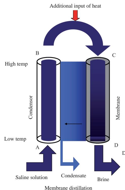
Fig. 4. Principle of membrane distillation (Memstill, TNO, The Netherlands; adapted).
