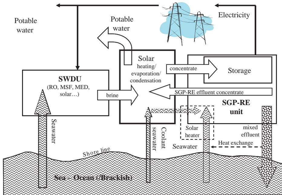
Fig. 1. Hybrid combination of solar energy, SWDU and SGP-RED unit.
