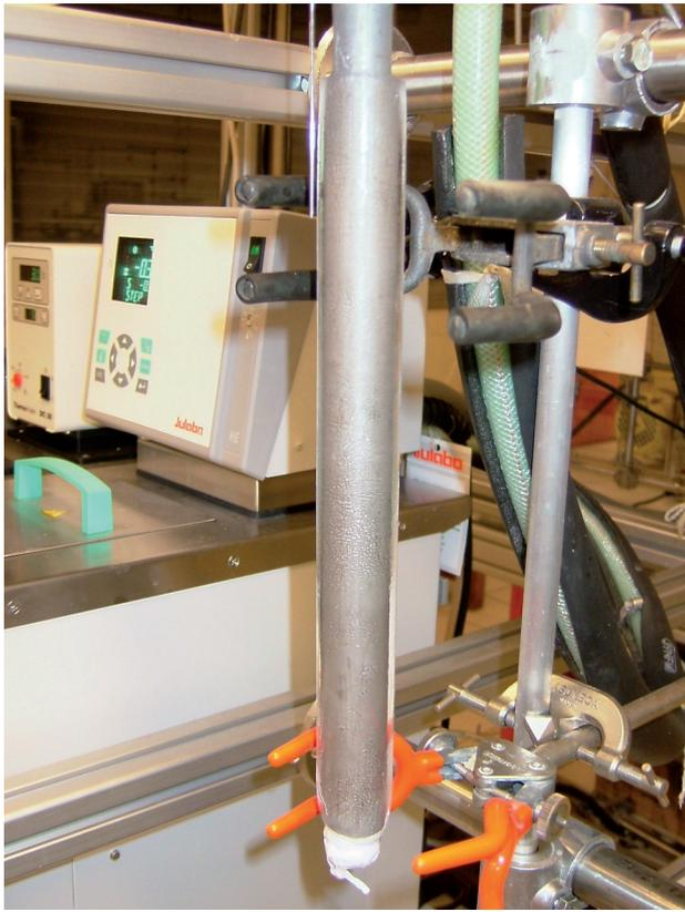
Fig. 6. Image of the ice of salinity 0.16 g/kg recovered in the 2nd stage of sea water desalination (run 48).
