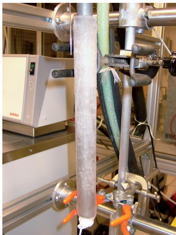
Fig. 5. Image of the ice of salinity 6.82 g/kg recovered in the 1st stage of sea water desalination (run 45).
