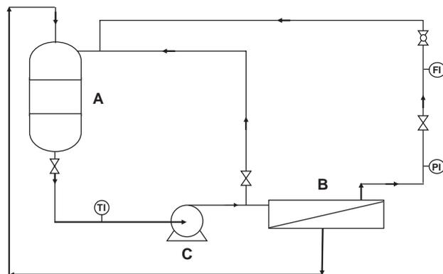
Fig. 1. Schematic flow diagram of nanofiltration test unit (flat membrane module): (A) feed tank, (B) membrane module, (C) pressure pump.
