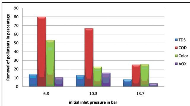
Fig. 8. Percentage removal of pollutants at different initial inlet pressure in the ultrafiltration treatment of combined bleach plant effluent.
