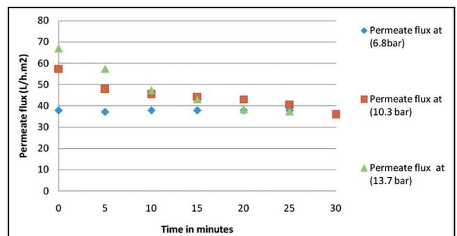
Fig. 3. Pattern of permeate flux in different initial inlet pressure (UF).
