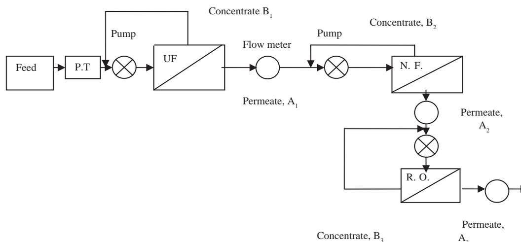
Fig. 1. Scheme of Pilot membrane treatment plant. Abbreviations: P.T.: primary treatment unit, UF: ultrafiltration, NF: nanofiltration, RO: reverse osmosis.
