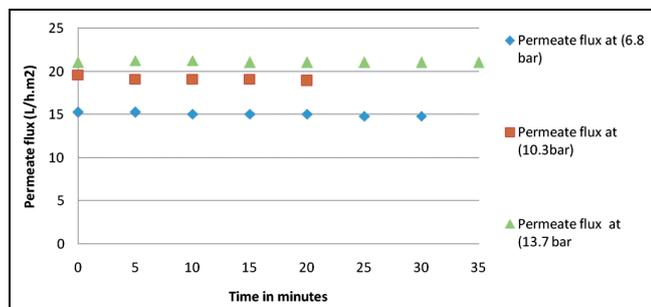
Fig. 5. Pattern of permeate flux in different initial inlet pressure (NF).
