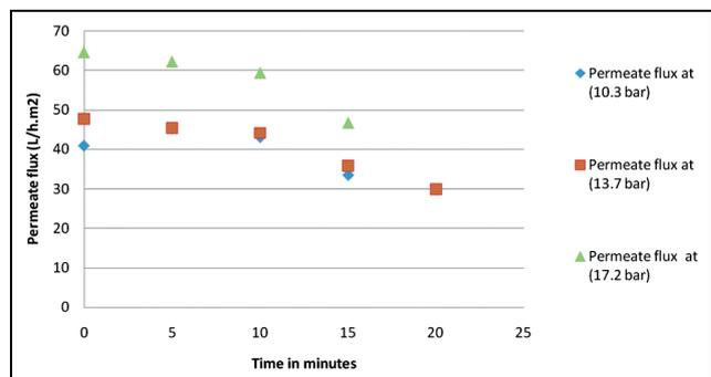
Fig. 7. Pattern of permeate flux in different initial inlet pressure (RO).
