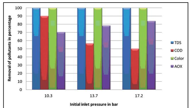
Fig. 10. Percentage removal of pollutants at different initial inlet pressure in the reverse osmosis treatment of combined bleach plant effluent.
