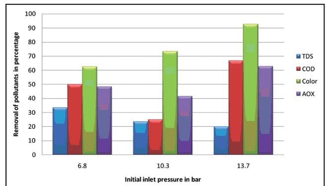
Fig. 9. Percentage removal of pollutants at different initial inlet pressure in the nanofiltration treatment of combined bleach plant effluent.
