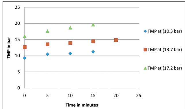
Fig. 6. Pattern of TMP in different initial inlet pressure (RO).
