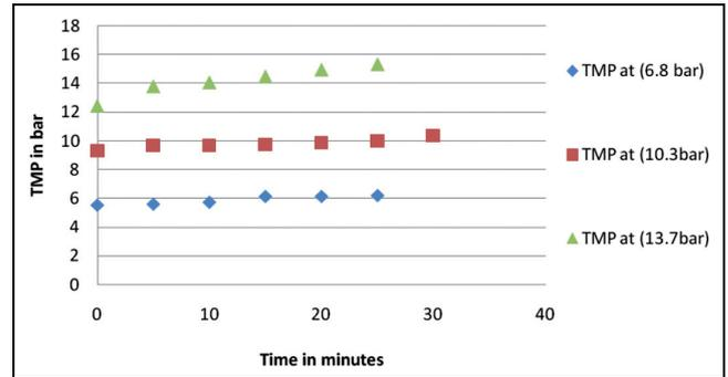
Fig. 2. Pattern of TMP in different initial inlet pressure (UF).
