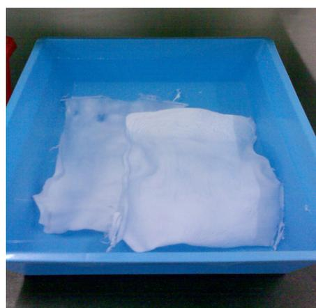
Fig. 1. Immersing of membranes in distilled water.
