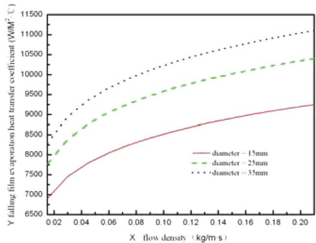
Fig. 5. Effect of flow density on the falling film evaporation heat transfer coefficient.
