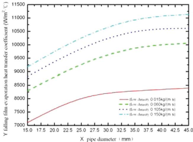
Fig. 8. Effect of pipe diameter on the falling film evaporation heat transfer coefficient; vacuum 0.05 MPa.
