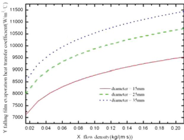
Fig. 3. Effect of vacuum on the falling film evaporation heat transfer coefficient; vacuum 0.05 MPa.
