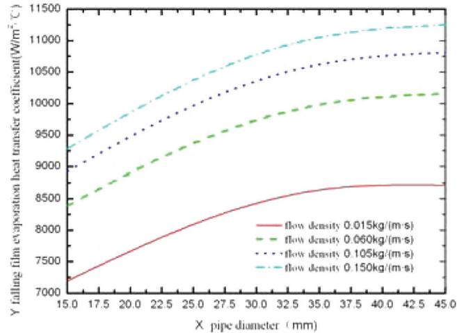
Fig. 9. Effect of pipe diameter on the falling film evaporation heat transfer coefficient; vacuum 0.07 MPa.
