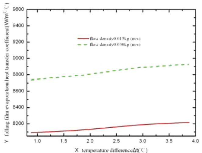
Fig. 6. Effect of temperature difference on the falling film evaporation heat transfer coefficient.
