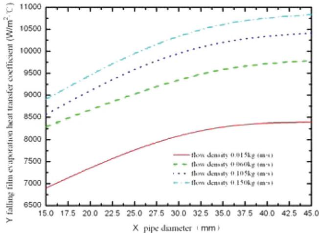
Fig. 7. Effect of pipe diameter on the falling film evaporation heat transfer coefficient; vacuum 0.03 MPa.
