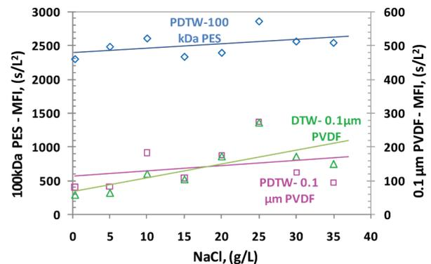
Fig. 10. MFI-UF at different addition of ionic strength of NaCl for 0.1 µm PVDF and 100 kDa PES at  $P = 1$  bar.
