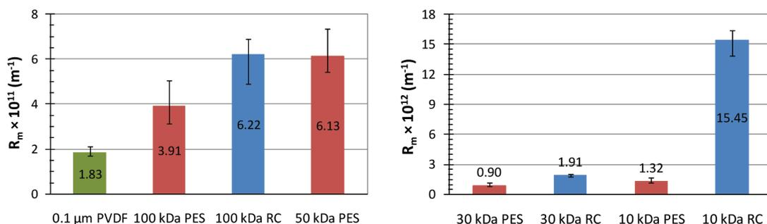
Fig. 3. Membrane resistance ( $R_m$ ) for the membranes tested in the study.
