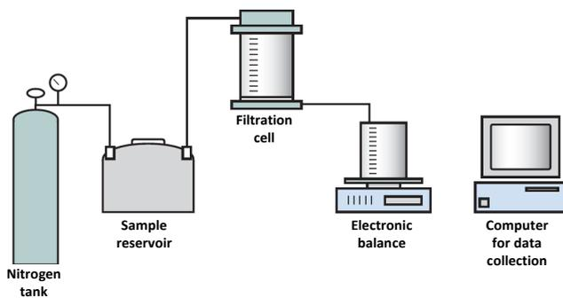
Fig. 2. Scheme of filtration setup [13].
