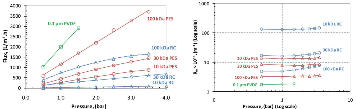
Fig. 4. Flux vs. pressure (left) and log plot of  $R_m$  vs. pressure (right) — RC and PES membranes.
