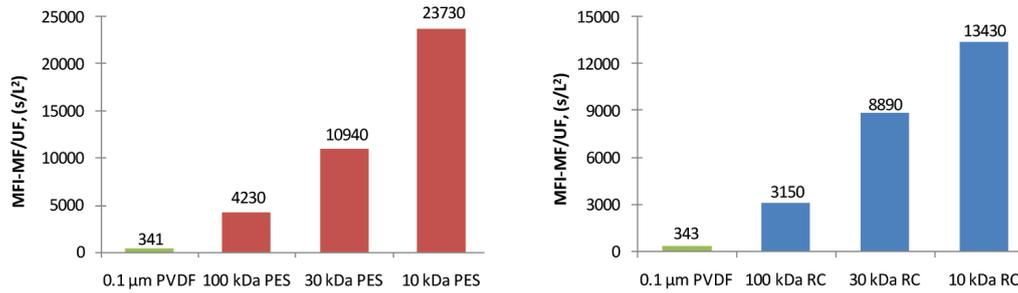
Fig. 11. MFI-UF values for pre-filtered (0.45 µm) North Sea water as function of MWCO and membrane material.
