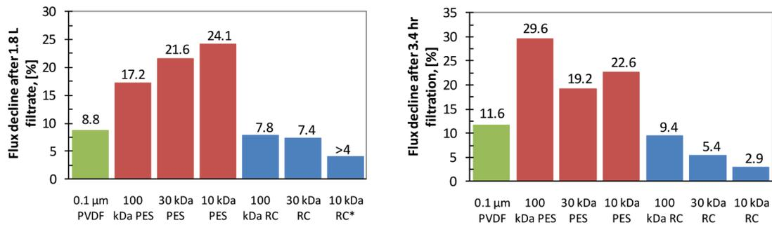
Fig. 8. Flux decline in % at same filtered volume (left) and at same exposure time (right) vs. membrane type.
