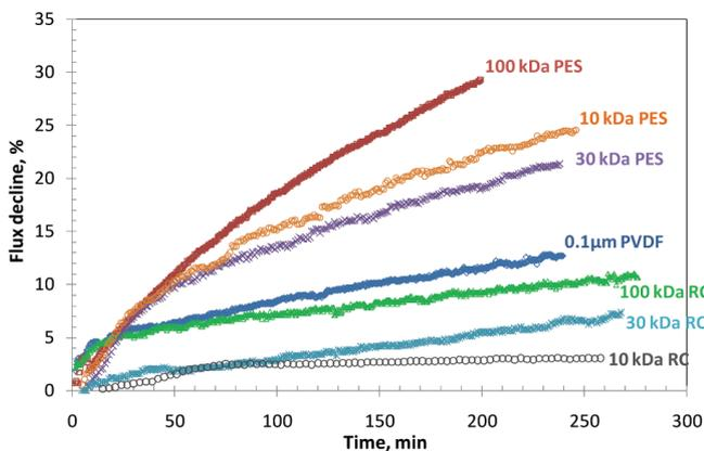
Fig. 6. Flux decline vs. filtration time (milli-Q + NaCl 35 g/L)..
