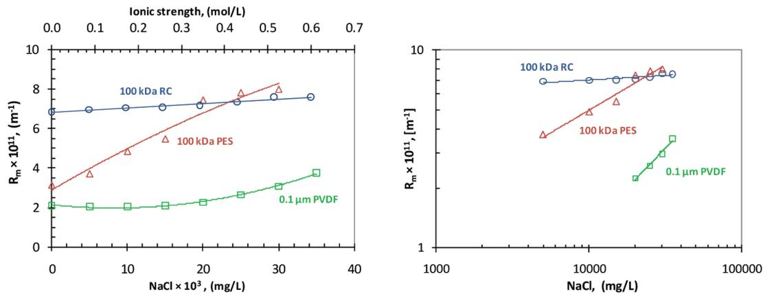
Fig. 5.  $R_m$  vs. ionic strength ( $P = 1$  bar) (left) and log plot  $R_m$  vs. log NaCl concentration (right).
