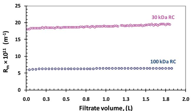
Fig. 7.  $R_m$  vs. filtrate volume for PES, RC and PVDF membranes (milli-Q + NaCl 35 g/L).
