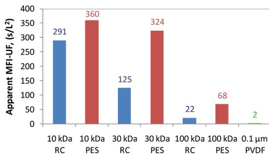
Fig. 9. Apparent MFI-UF after filtration with milli-Q + NaCl (35 g/L).
