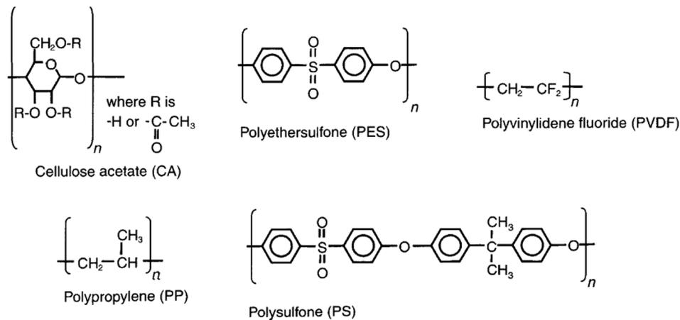
Fig. 1. Chemical structure of common MF/UF membrane materials [12].
