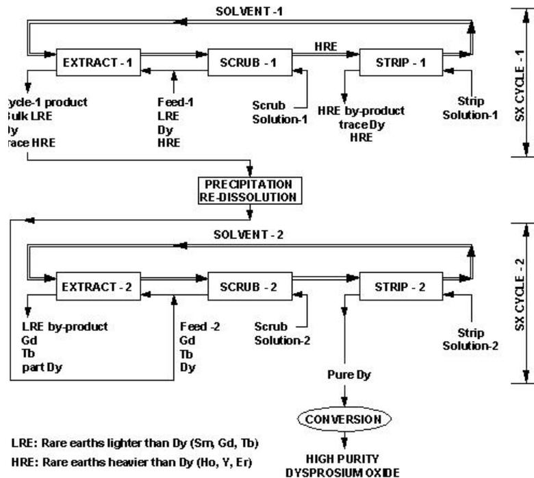
Fig. 1. Generic dual cycle solvent extraction separation process for dysprosium purification.
