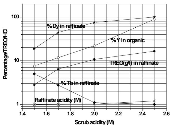
Fig. 5. Effect of scrub acidity on purity of Dy.
