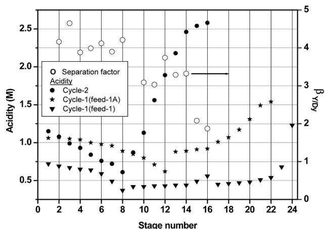
Fig. 2. Stage to stage variation of acidity and separation factor.
