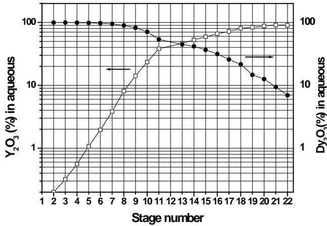
Fig. 3. Stage to stage variation of Dy and Y in cycle-1.
