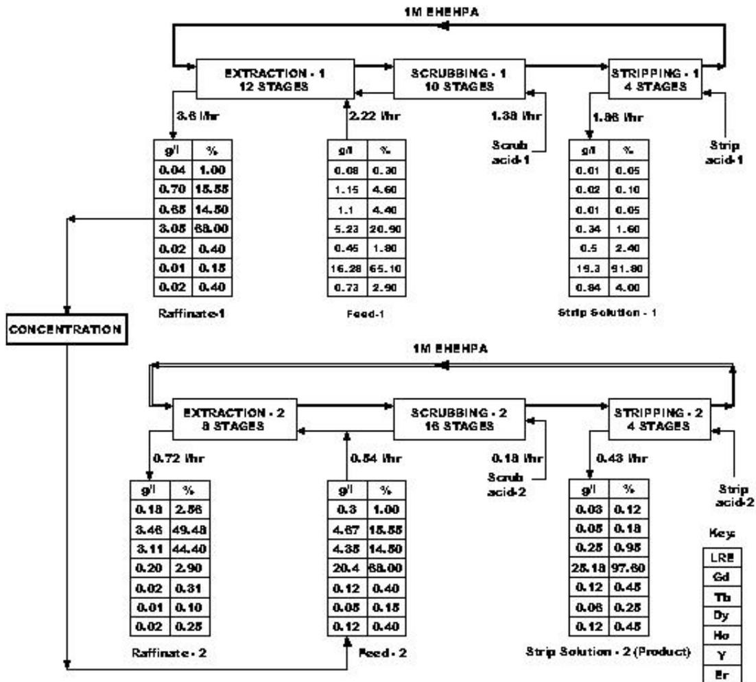
Fig. 4. Material balance for 54-stage mixer settler cascade for separation of high purity  $Dy_2O_3$ .
