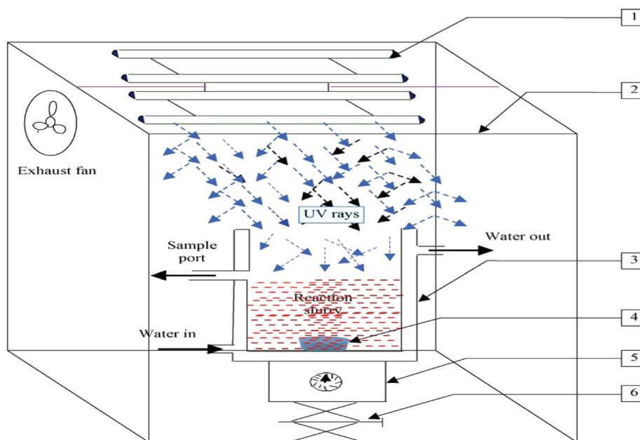
Fig. 1. Experimental setup for photocatalytic process. 1, UV lamps-5 (30 W); 2, chamber; 3, jacketed reactor; 4, magnetic bead; 5, magnetic stirrer; 6, lab jack.
