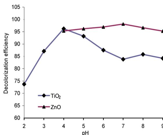
Fig. 3. Effect of pH on degradation of malachite green (50 ppm MG; 1 g/l catalyst; time 2.5 h).
