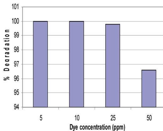
Fig. 4. Effect of MG concentration on degradation (1 g/l TiO<sub>2</sub>; time 2 h).
