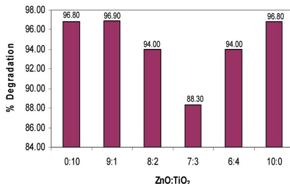
Fig. 2. Effect of variation of ratios of catalyst on degradation of malachite green (50 ppm MG; time of reaction 2 h).
