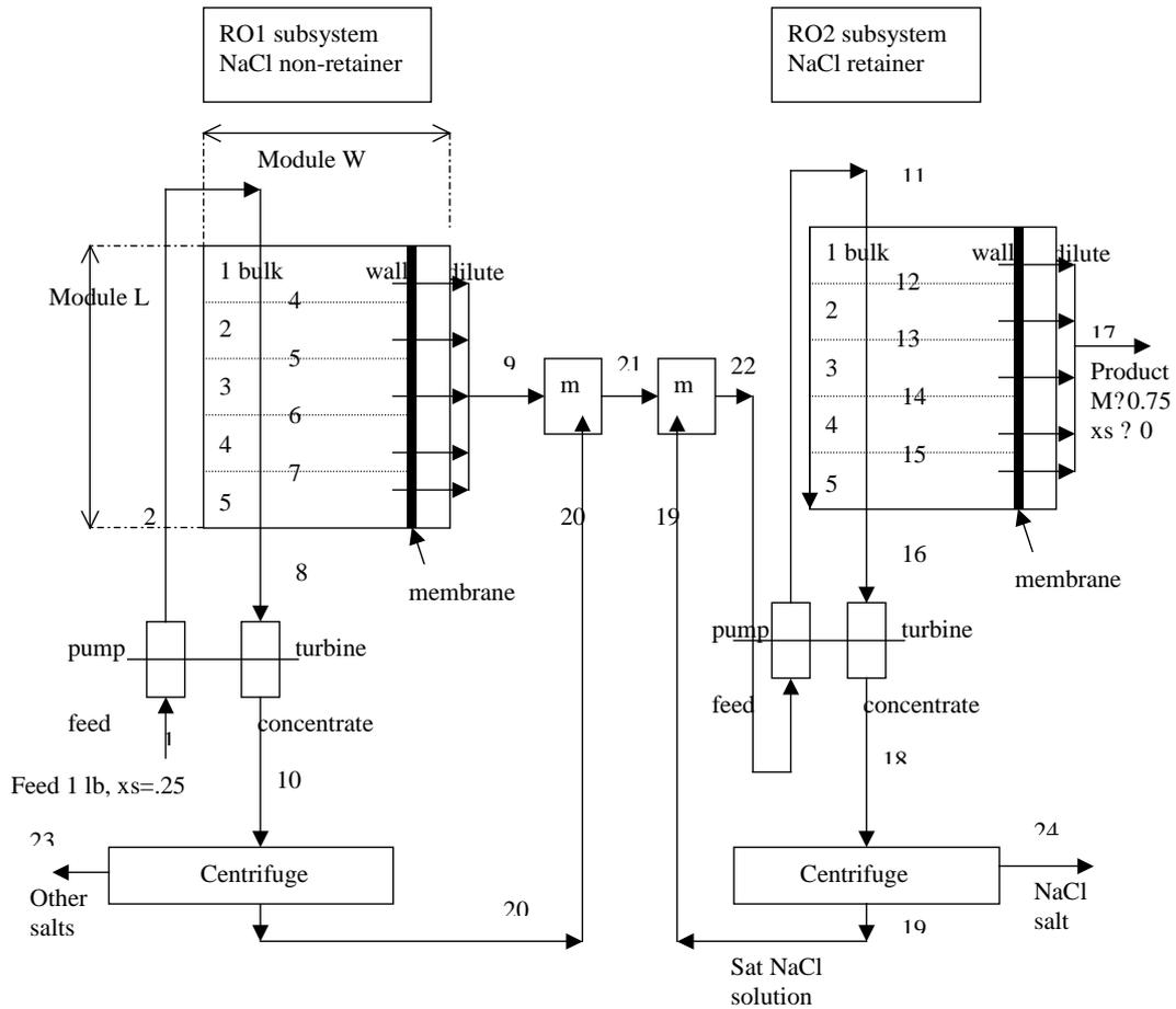
Fig. 6. A concept of RO for zero liquid discharge.
