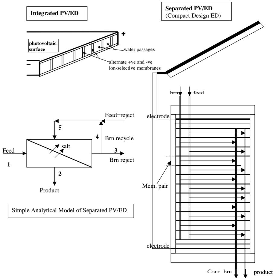
Fig. 8. The photovoltaic/electrodialysis (PV/ED).
