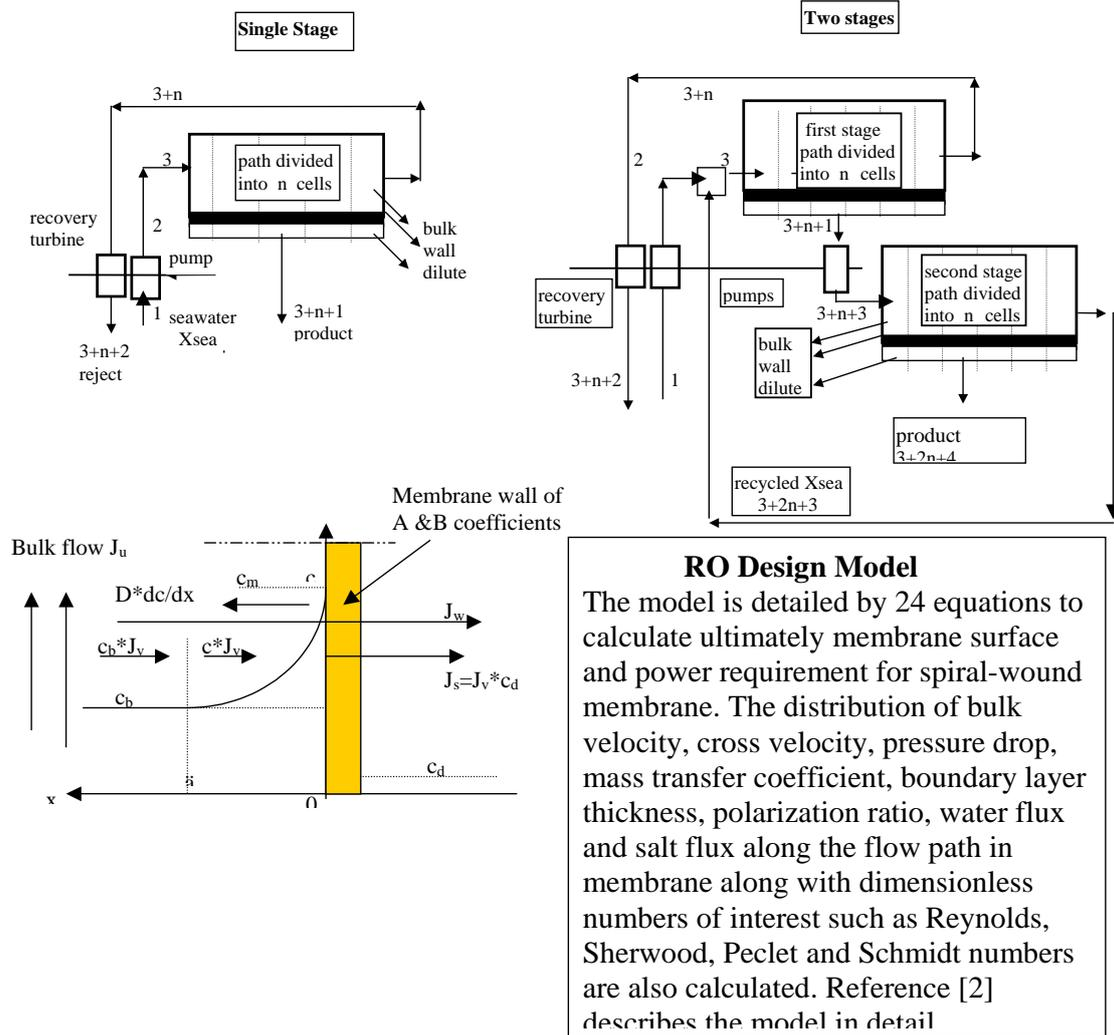
Fig. 5. The reverse osmosis desaliner (RO) [1,2].
