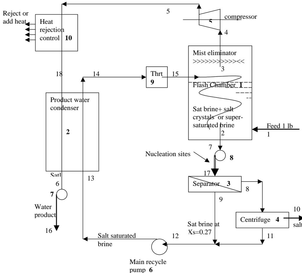
Fig. 4. VC for zero liquid discharge (ZLD).
