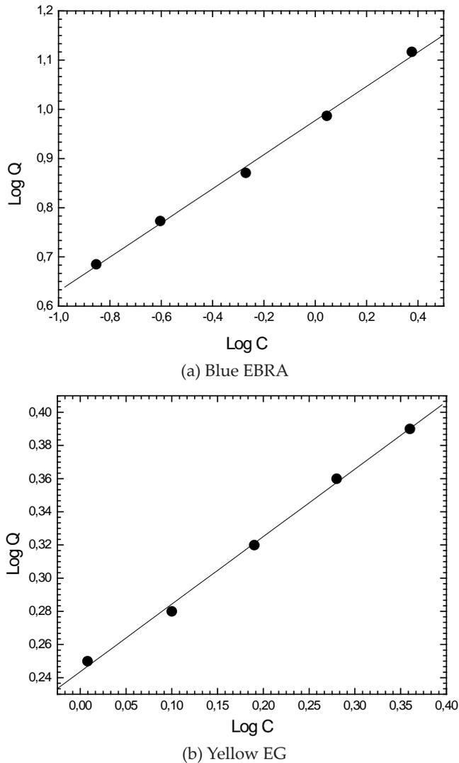
Fig. 10. Adsorption of residual dye concentration on PAC. Modeling by a Freundlich equation.
