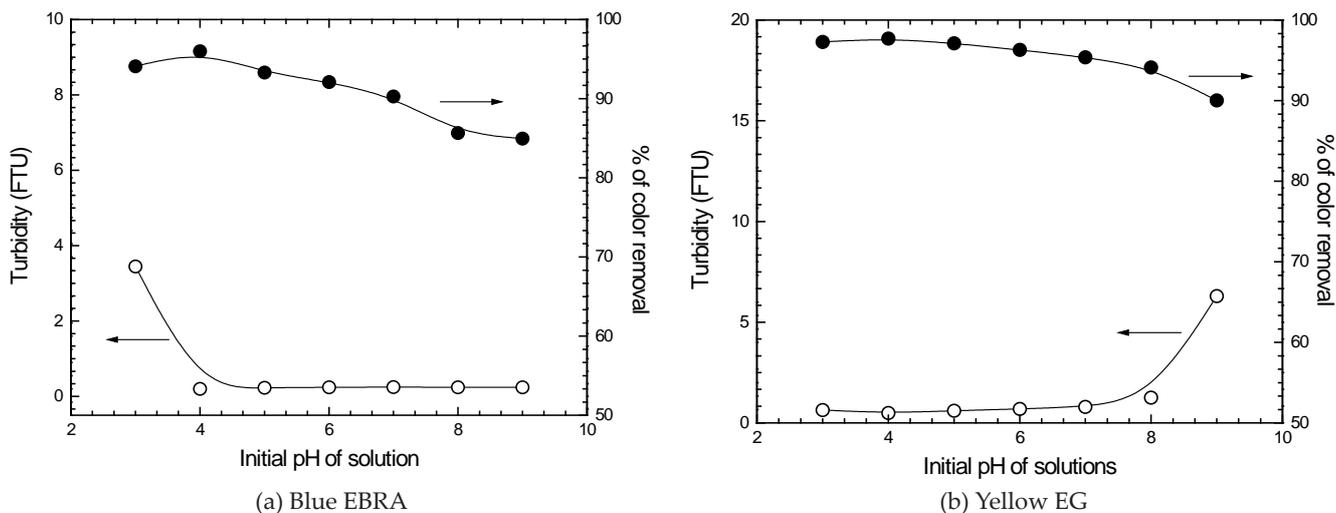
Fig. 6. Coagulation–flocculation of dyes by PAH/bentonite at optimal doses of PAH. Turbidity and color removal as functions of initial pH of solutions.  $V_{\text{sample}} = 500 \text{ mL}$ ;  $C_0 = 100 \text{ mg/L}$ ;  $V_{\text{PAH}} = 5.1 \text{ mL}$  (a) and  $2.7 \text{ mL}$  (b);  $T = 20^\circ\text{C}$ .
