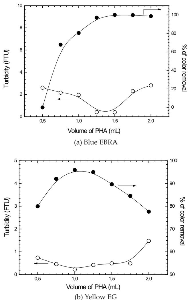
Fig. 3. Coagulation–flocculation of dyes by PAH/bentonite. Turbidity and color removal as functions of volume of PAH.  $V_{\text{sample}} = 500$  mL;  $C_0 = 20$  mg/L;  $m_{\text{bentonite}} = 75$  mg;  $\text{pH}_i = 7 \pm 0.05$ ;  $T = 20^\circ\text{C}$ .
