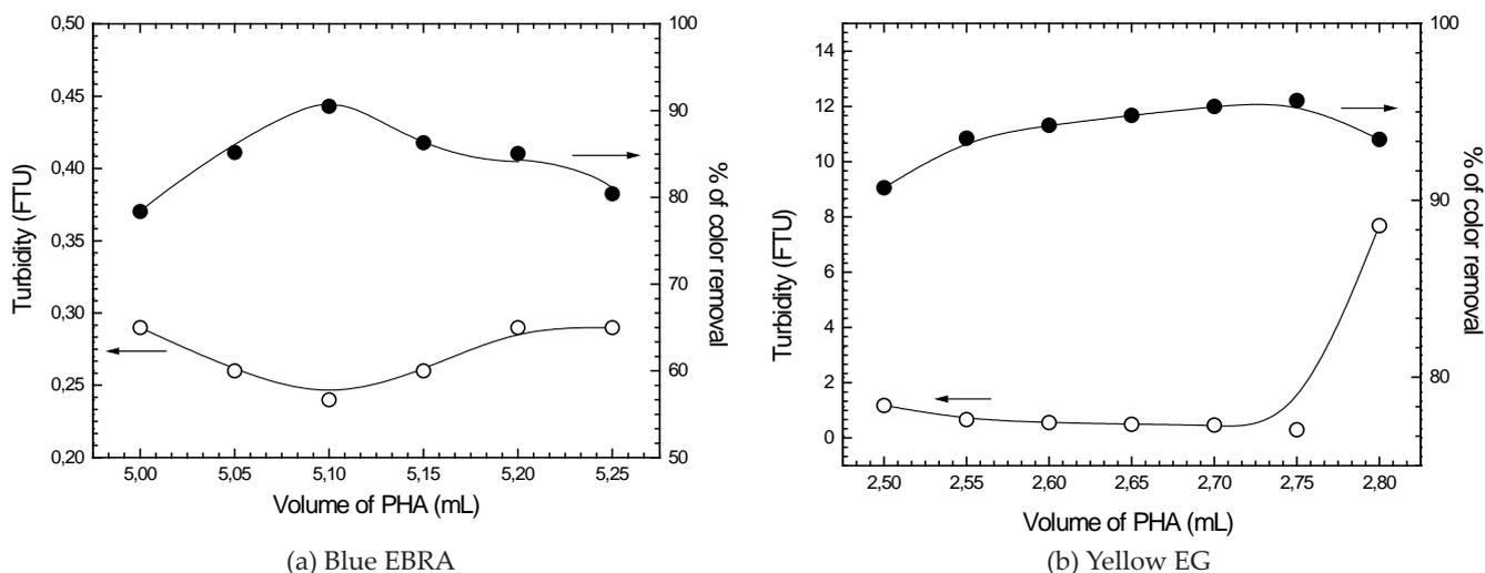
Fig. 5. Coagulation–flocculation of dyes by PAH/bentonite. Turbidity and color removal as functions of volume of PHA.  $V_{\text{sample}} = 500 \text{ mL}$ ;  $C_0 = 100 \text{ mg/L}$ ;  $m_{\text{bentonite}} = 250 \text{ mg}$  (a) and  $187.5 \text{ mg}$  (b);  $pH_1 = 7 \pm 0.05$ ;  $T = 20^\circ\text{C}$ .
