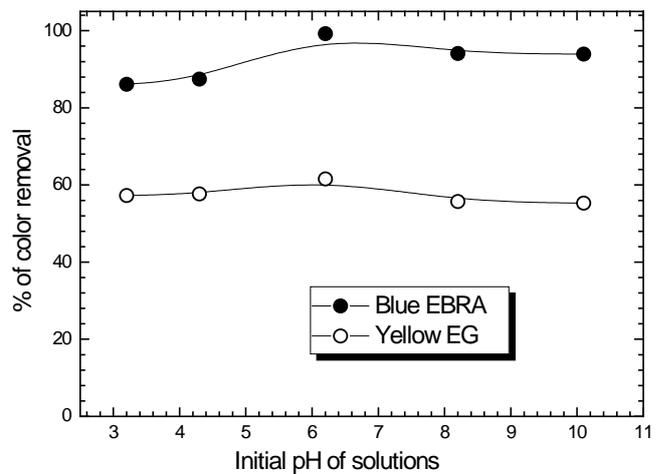
Fig. 8. Adsorption of residual dye concentration on PAC. Color removal as a function of initial pH of solutions.  $V_{\text{sample}} = 100$  mL;  $C_{\text{Ro(EBRA)}} = 4.85$  mg/L;  $C_{\text{Ro(EG)}} = 2.82$  mg/L;  $m_{\text{PAC}} = 100$  mg;  $T = 25^\circ\text{C}$ ; Agit. = 300 rpm; Contact time = 24 h.
