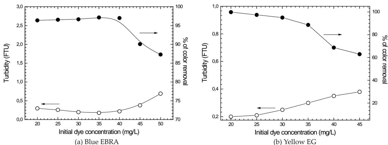
Fig. 4. Coagulation–flocculation of dyes by PAH/bentonite at optimal doses of PAH. Turbidity and color removal as functions of initial dye concentration.  $V_{\text{sample}} = 500 \text{ mL}$ ;  $m_{\text{bentonite}} = 75 \text{ mg}$ ;  $V_{\text{PHA}} = 1.5 \text{ mL}$  (a) and  $1.0 \text{ mL}$  (b);  $pH_1 = 7 \pm 0.05$ ;  $T = 20^\circ\text{C}$ .
