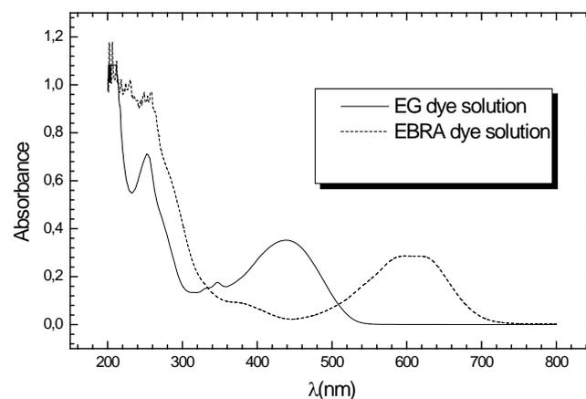
Fig. 2. UV spectra of 100-mg/L EBRA and EG dye solutions.
