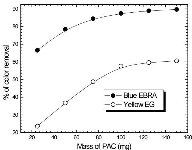
Fig. 7. Adsorption of residual dye concentration on PAC. Color removal as a function of the mass of PAC.  $V_{\text{sample}} = 100 \text{ mL}$ ;  $C_{\text{Ro(EBRA)}} = 4.85 \text{ mg/L}$ ;  $C_{\text{Ro(EG)}} = 2.82 \text{ mg/L}$ ;  $\text{pH}_i = 4.30 \pm 0.05$ ;  $T = 25^\circ\text{C}$ ; Agit. = 300 rpm; Contact time = 24 h.
