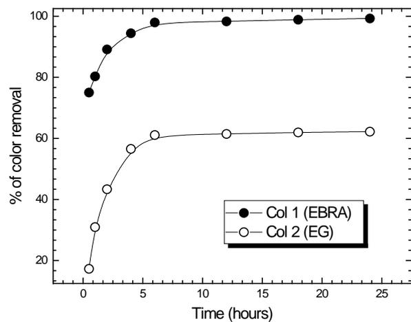
Fig. 9. Adsorption of residual dye concentration on PAC. Color removal as a function of contact time.  $V_{\text{sample}} = 100$  mL;  $C_{\text{Ro(EBRA)}} = 4.85$  mg/L;  $C_{\text{Ro(EG)}} = 2.82$  mg/L;  $\text{pH}_i = 6 \pm 0.05$ ;  $m_{\text{PAC}} = 100$  mg;  $T = 25^\circ\text{C}$ ; Agit. = 300 rpm.
