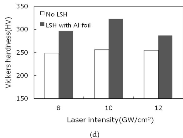
Fig. 6. Photographs of the sample coated with Al foil (a) before and (b) after laser shock hardening, (c) scanning electron microscope image of the surface of a laser shock hardened sample, and (d) measured Vickers hardness for different laser intensities.
