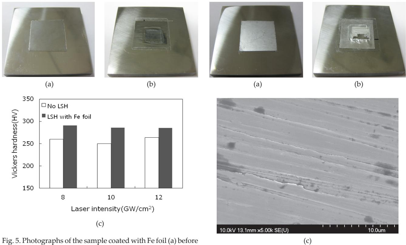
Fig. 5. Photographs of the sample coated with Fe foil (a) before and (b) after laser shock hardening and (c) measured Vickers hardness for different laser intensities.
