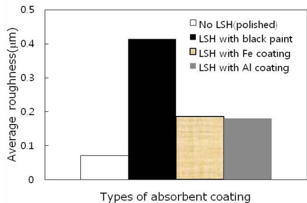
Fig. 4. Surface roughness of laser shock hardened samples with various coatings (sample surface was polished).
