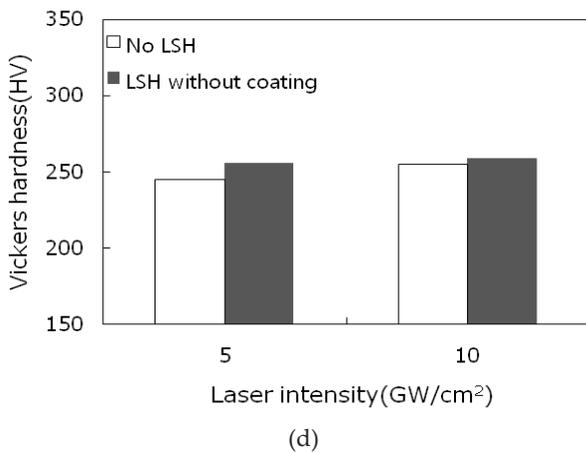
Fig. 3. Photographs of the sample coated with black paint (a) before and (b) after laser shock hardening and (c) measured Vickers hardness for different laser intensities.
