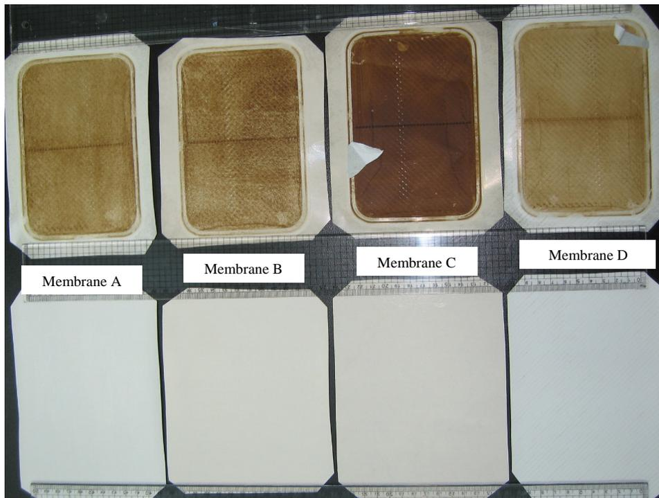
Fig. 1. Images of membranes before (below images) and after (upper images) the fouling test.
