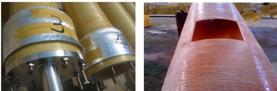
Fig. 7. Pipes made by different winding angles.
