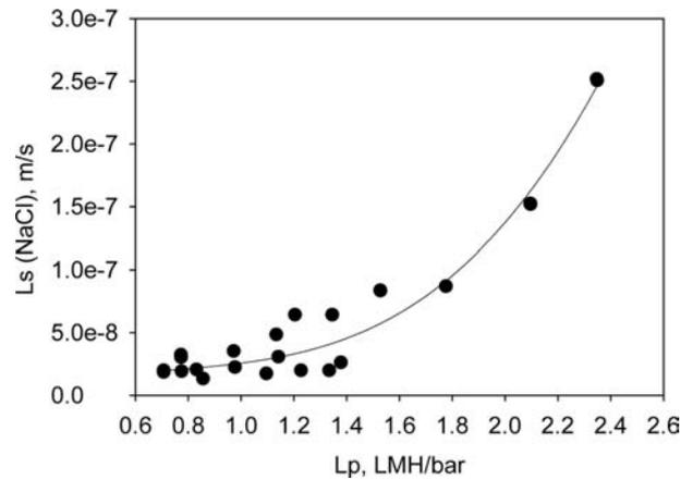
Fig. 1. Correlation between  $L_p$  and  $L_s$  (NaCl).
