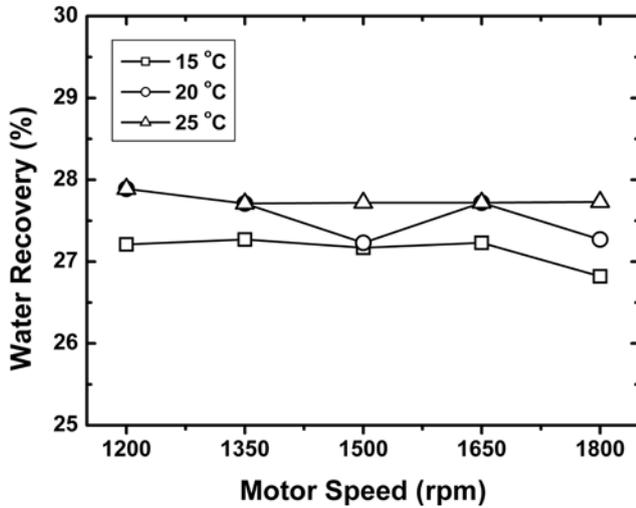
Fig. 7. Water recovery ratio in response to the motor speed and feedwater temperature.
