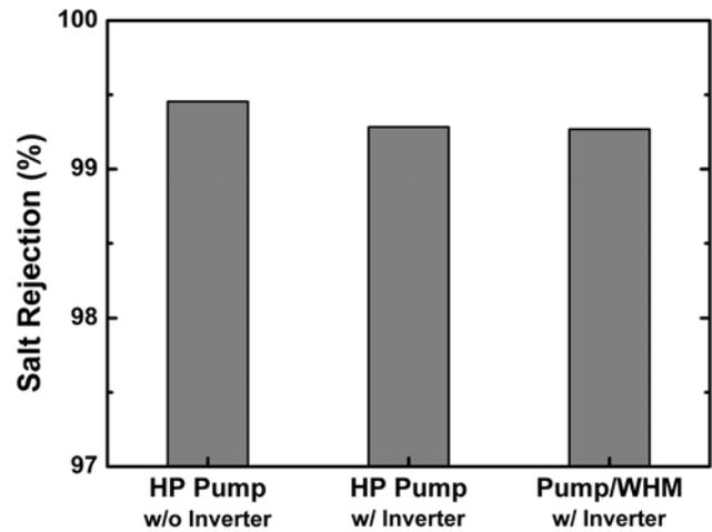
Fig. 11. Effect of the water hydraulic motor (WHM) as an energy recovery device on salt rejection.
