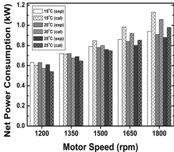
Fig. 6. Calculated net power consumption and measured net power consumption in response to the motor speed.
