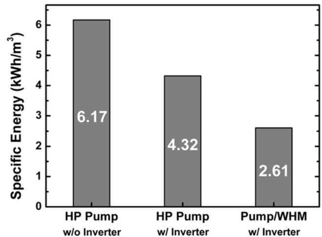
Fig. 9. Effect of water hydraulic motor (WHM) as energy recovery device on specific energy consumption.
