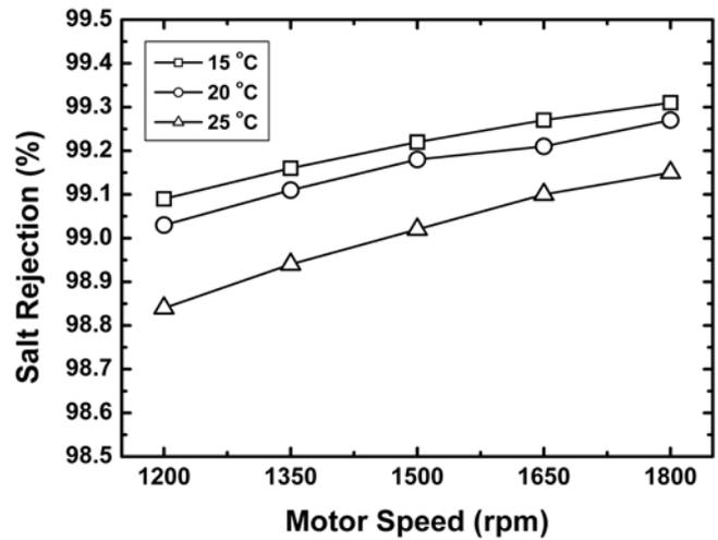
Fig. 8. Salt rejection in response to the motor speed and feedwater temperature.
