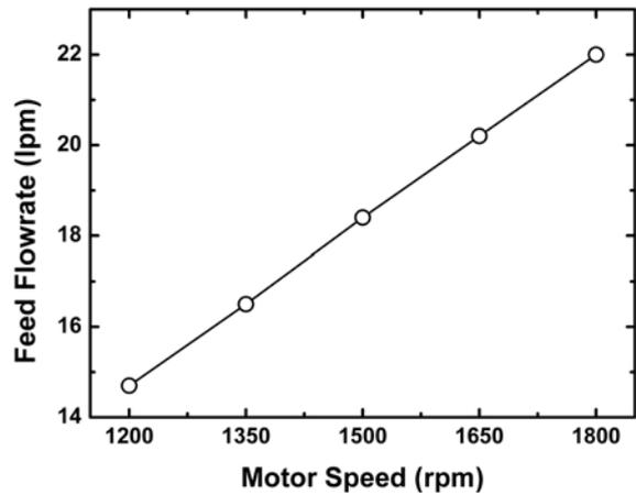
Fig. 4. Change of feedwater flowrate in response to the motor speed.
