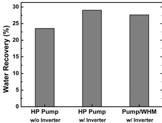
Fig. 10. Effect of the water hydraulic motor (WHM) as an energy recovery device on water recovery ratio.
