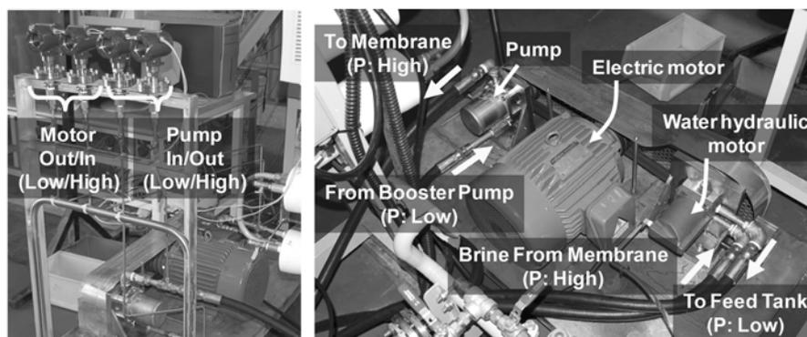
Fig. 2. Photographs of the water hydraulic pump-motor assembly.
