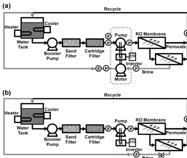
Fig. 1. Schematic diagrams of experimental setup. (a) RO system equipped with water hydraulic pump-motor assembly, (b) RO system equipped with a conventional high-pressure pump.
