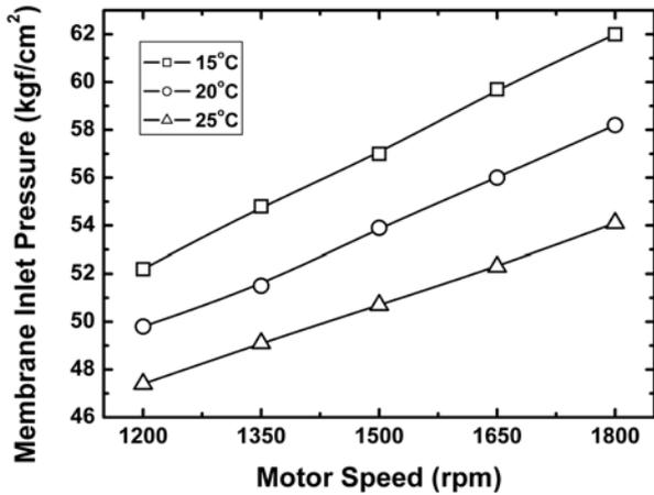
Fig. 3. Change of membrane inlet pressure in response to the motor speed and feedwater temperature.
