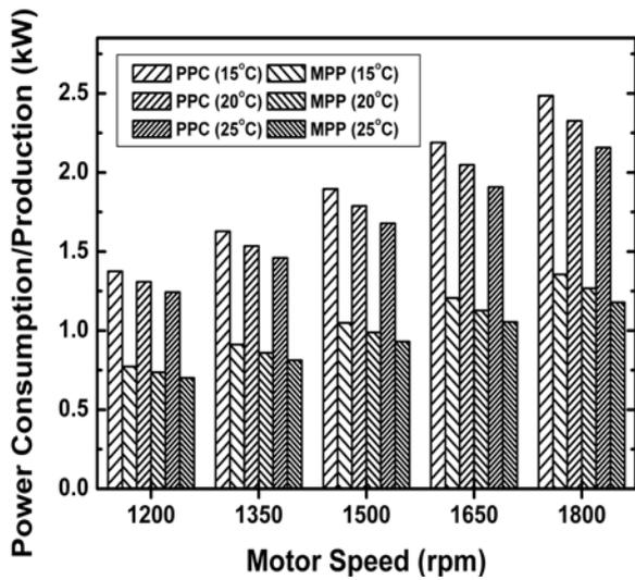
Fig. 5. Calculated pump power consumption (PPC) and calculated motor power production (MPP) in response to the motor speed. Here, the motor means the water hydraulic motor for energy recovery.
