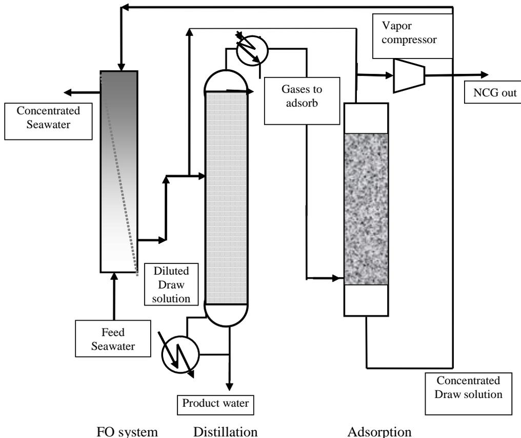
Fig. 1. Basic sections in forward desalination.
