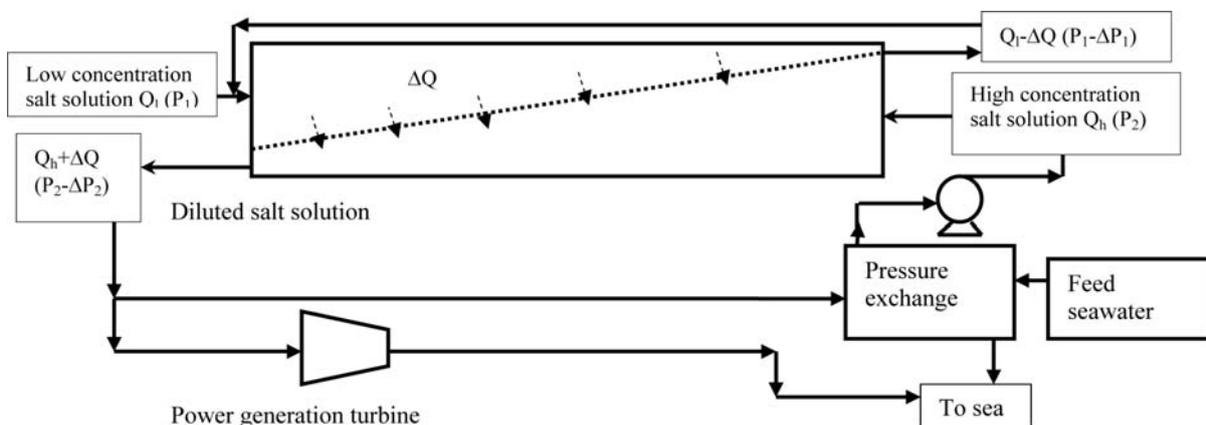
Fig. 2. Block diagram for osmosis energy generation.
