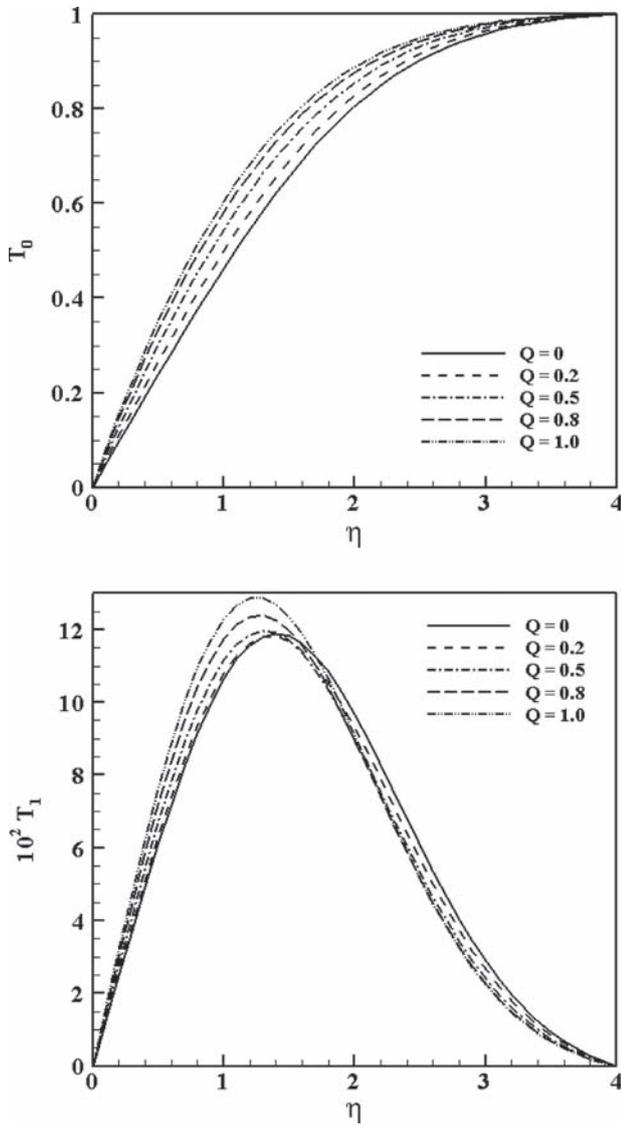
Fig. 5. Temperature profiles with the variation of  $Q$  for  $P = 0.71, M = 0.5, K = 3, N = 0.5$ .
