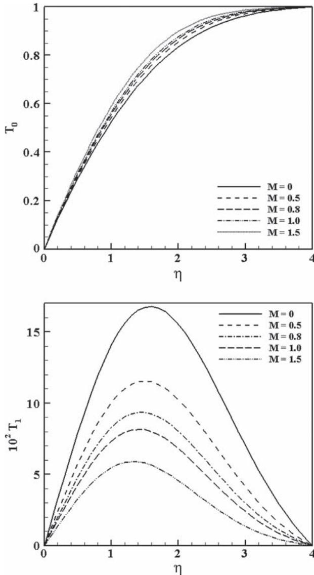
Fig. 3. Temperature profiles with the variation of  $M$  for  $P = 0.71, N = 0.5, K = 3, Q = 0.5$ .
