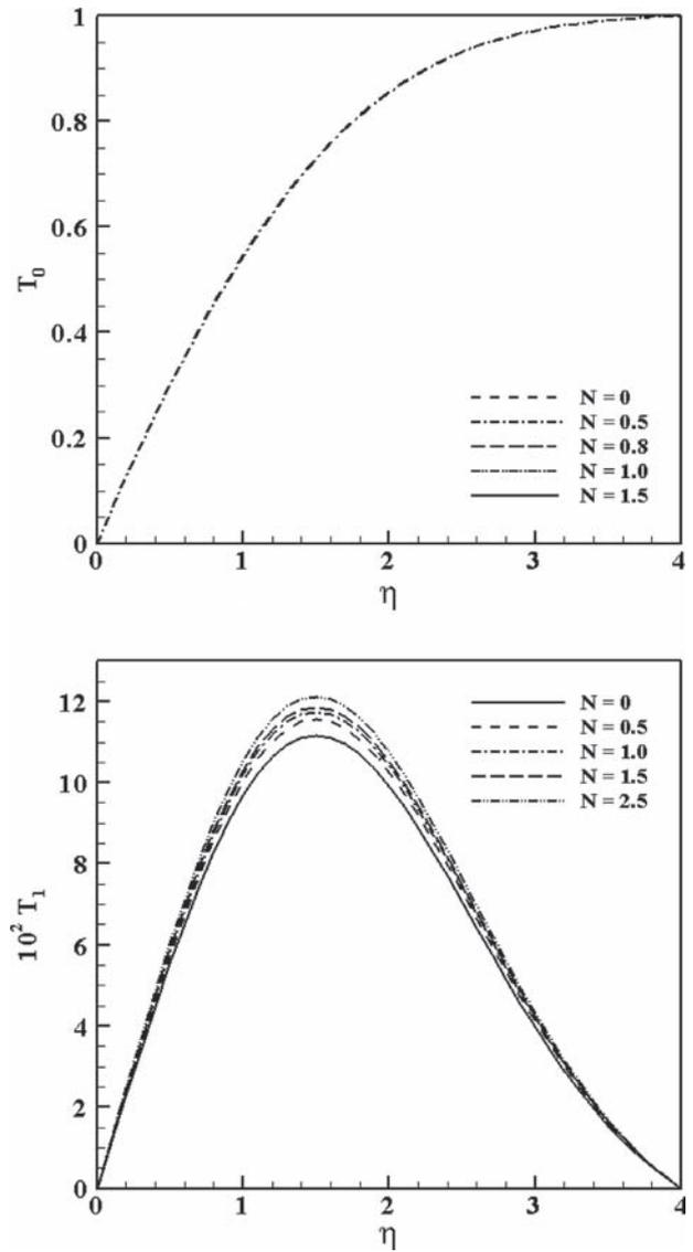
Fig. 4. Temperature profiles with the variation of  $N$  for  $P = 0.71, M = 0.5, K = 3, Q = 0.5$ .
