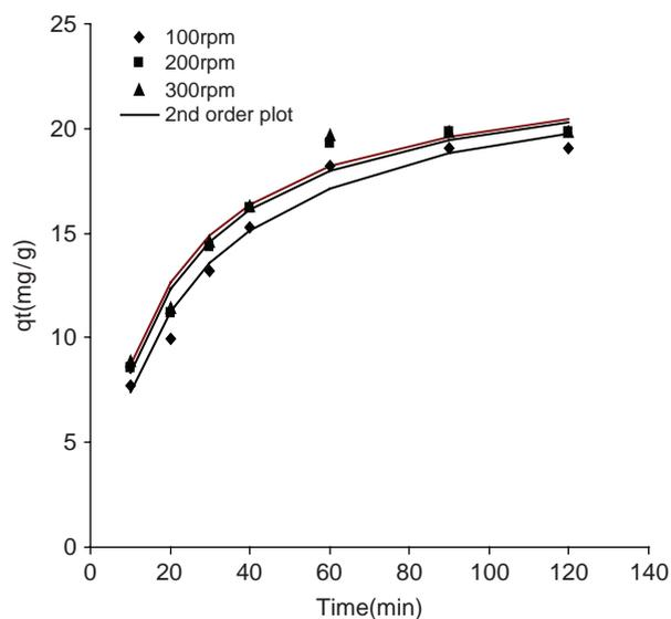
Fig. 4. Comparison of pseudo-second-order kinetic model in predicting  $q$  (mg/g) for Cu ion sorption at different agitation speed.
