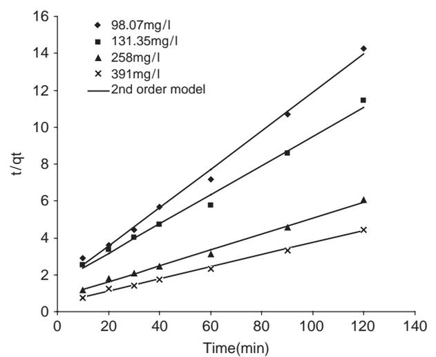
Fig. 2. Applicability of pseudo-second-order kinetic model to experimental data at different initial Cu (II) ion concentration.
