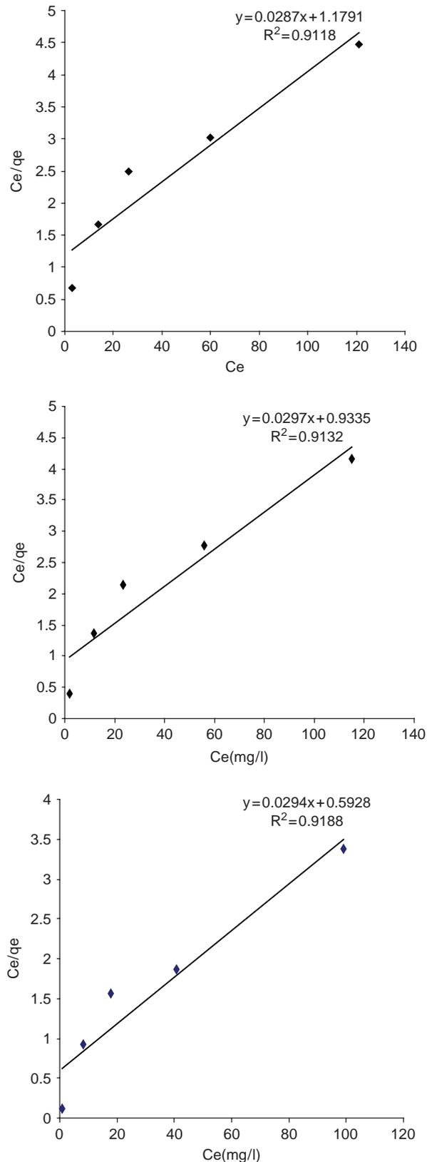
Fig. 7. Langmuir isotherm plot at different temperatures ( $a = 309$  K;  $b = 333$  K;  $c = 353$  K)
