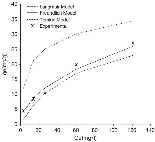
Fig. 6. Applicability of different isotherm plots to experimental data.
