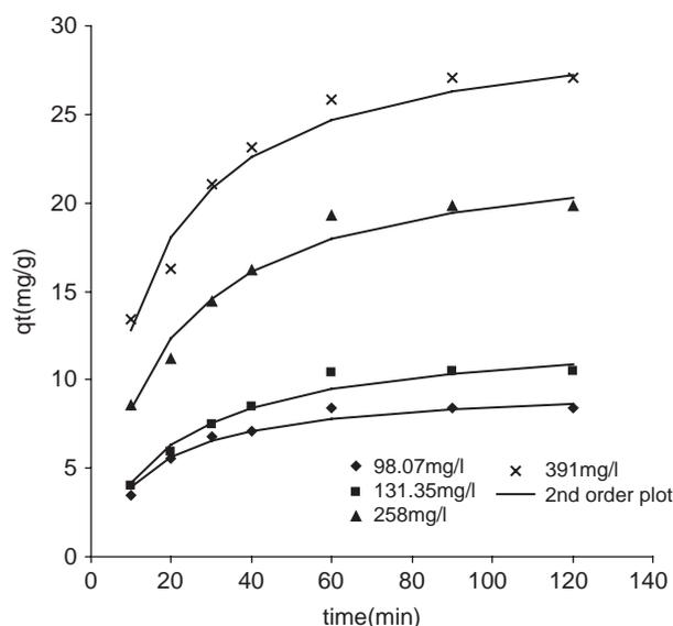
Fig. 1. Comparison of pseudo-second-order kinetic model in predicting  $q(\text{mg/g})$  for Cu ion sorption at different initial Cu (II) ion concentration.
