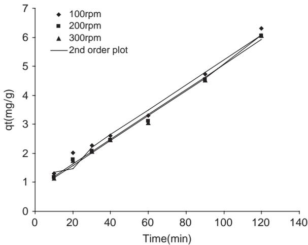
Fig. 5. Applicability of pseudo-second-order kinetic model to experimental data at different agitation speed.
