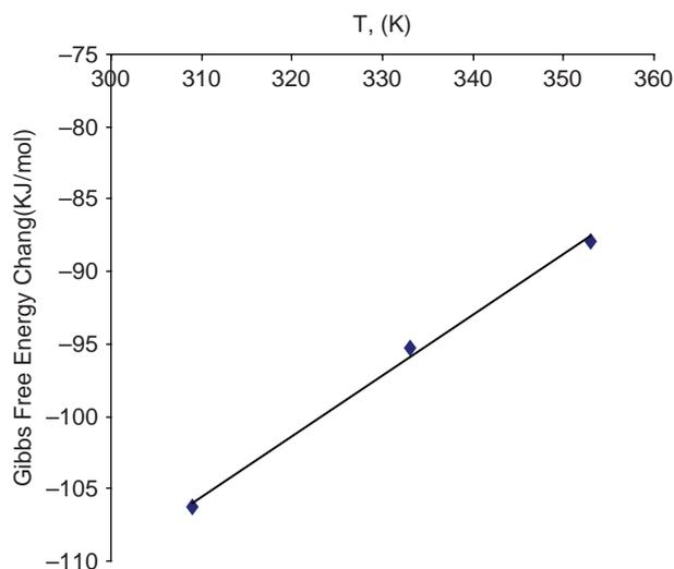
Fig. 8. Relationship between Gibbs free energy change ( $\Delta G^\circ$ ) and temperature (K) of sorption of Cu (II) ion by ST.
