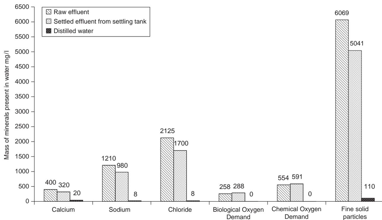
Fig. 2. Chemical analysis of raw effluent, settled effluent and distilled water.
