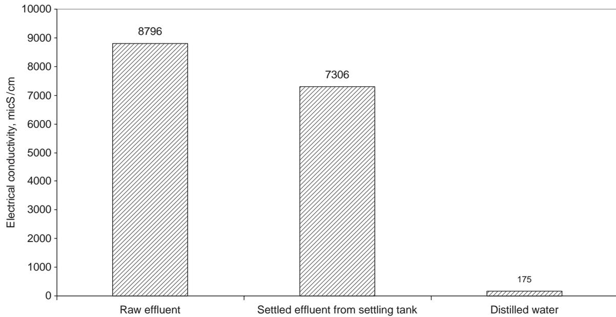
Fig. 3. Variation of electrical conductivity for various samples.
