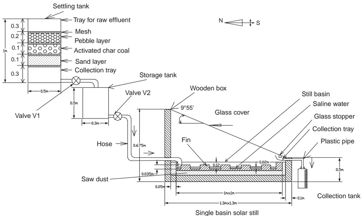
Fig. 1. Solar still integrated with an effluent settling tank.
