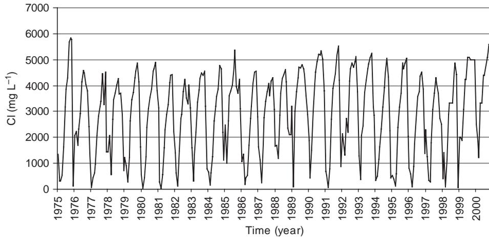
Fig. 3. Chloride concentration in Almyros springwater versus time (monthly measurements).
