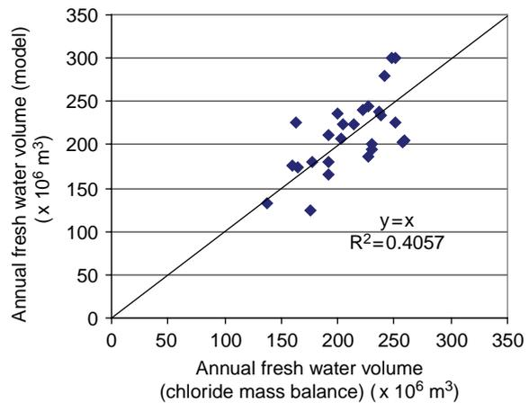
Fig. 6. Annual fresh water volumes calculated by the model versus the ones estimated by the chloride mass balance approach.
