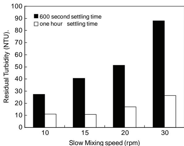
Fig. 5. Effect of slow mixing on removal of *Chlorella sp.* suspended in simulated seawater.
