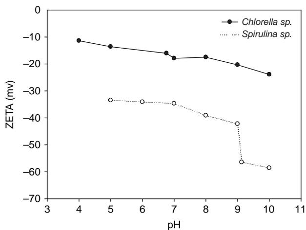
Fig. 9. Changes in surface zeta-potential at various solution pH values for *Chlorella sp.* and *Spirulina sp.*
