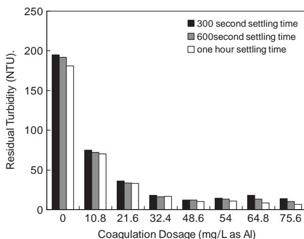
Fig. 10. Effect of coagulant dosage on removal of *Chlorella sp.* suspended in simulated seawater.
