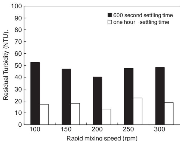
Fig. 4. Effect of rapid mixing on removal of *Chlorella sp.* suspended in simulated seawater.
