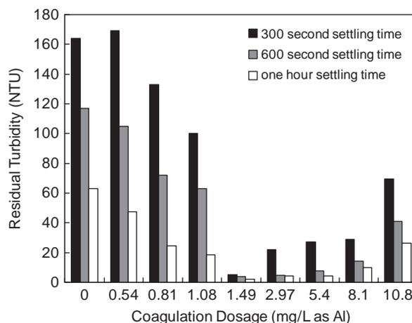
Fig. 2. Residual turbidity versus settling time for freshwater *Chlorella sp.* suspension coagulated with various coagulant dosages.
