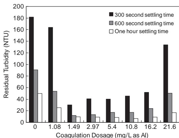
Fig. 3. Residual turbidity versus settling time for seawater *Chlorella sp.* suspension coagulated with various coagulant dosages.
