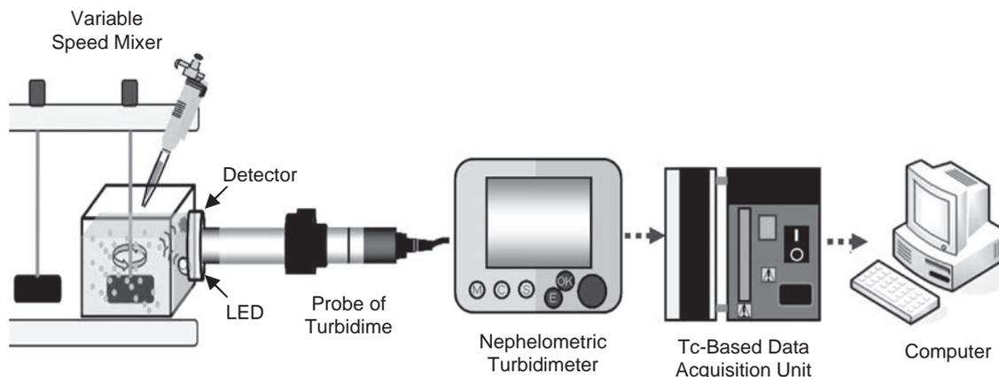
Fig. 1. Laboratory setup for conducting Jar test and continuously monitoring turbidity of coagulated algal solution.
