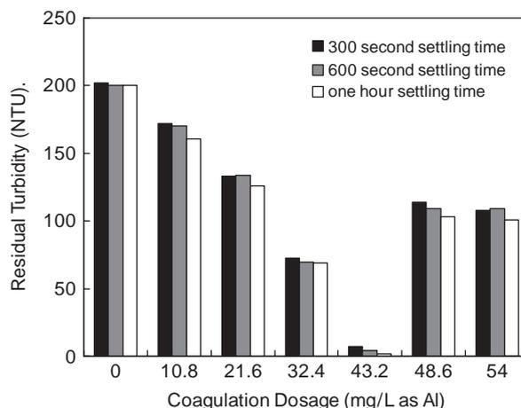
Fig. 6. Effect of coagulant dosage on removal of *Spirulina sp.* suspended in freshwater.
