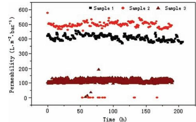
Fig. 8. Tendency of permeability of the UF membrane in the tests.
