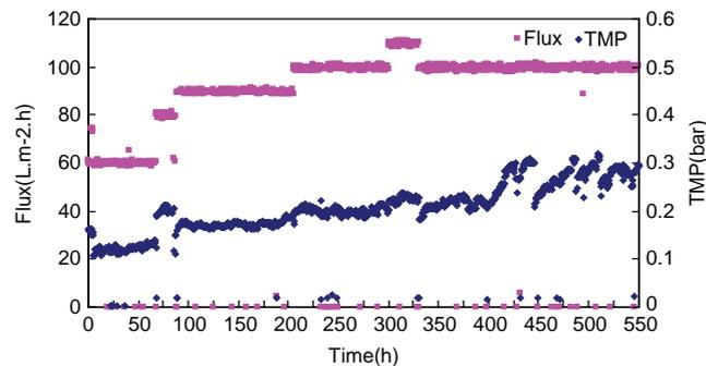
Fig. 6. Variation of flux and TMP of UF membrane on Sample 2 after coagulation.
