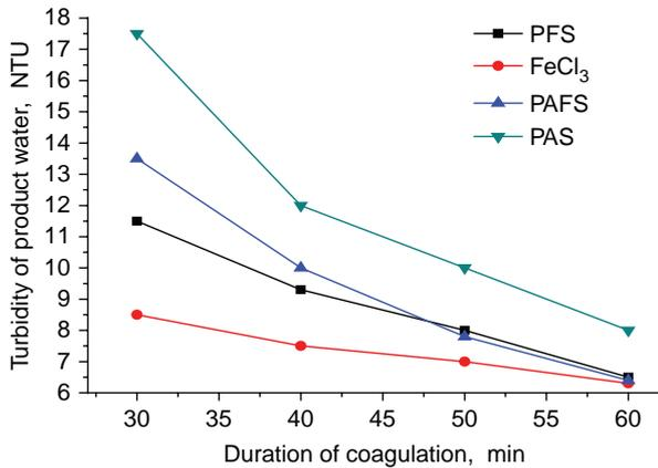
Fig. 2. Clarification effect of raw seawater treated with four types of coagulants.
