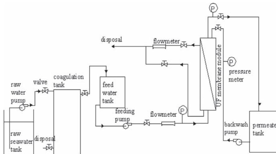
Fig. 1. Schematic diagram of the pilot scale test of UF system.
