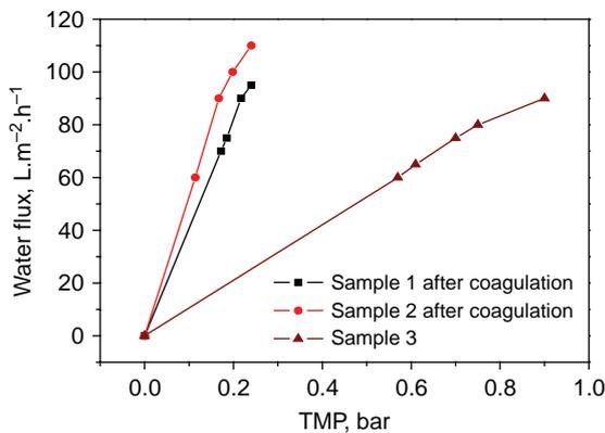
Fig. 4. Relationship between permeation flux and TMP of UF membrane fed with three different types of raw water.
