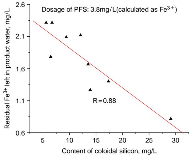
Fig. 3. Relationship between residual ferric in product water and the colloidal silicon in raw seawater.
