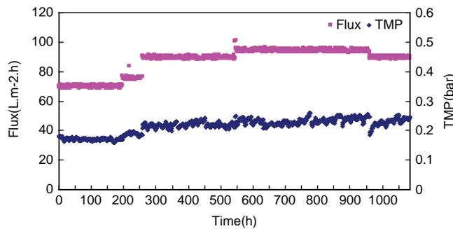
Fig. 5. Variation of flux and TMP of UF membrane on Sample 1 after coagulation.
