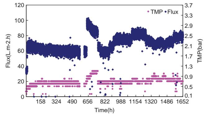
Fig. 7. Variation of flux and TMP of UF membrane on Sample 3 without coagulation.
