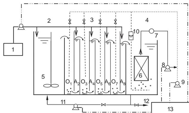
Fig. 1. Schematic diagram of the An-(O/A)<sup>n</sup>-MBR system. 1. Wastewater reservoir, 2. Anaerobic reactor, 3. Multiple phases of aerobic and anoxic zones, 4. MBR tank, 5. Agitator, 6. Membrane module, 7. Pressure gauge, 8. Peristaltic pump, 9. Air blower, 10. Air flow meter, 11. Return sludge, 12. Excess sludge, 13. PLC system.
