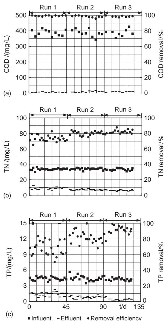
Fig. 2. Influent and effluent qualities and removal efficiency: (a) COD, (b) TN and (c) TP.
