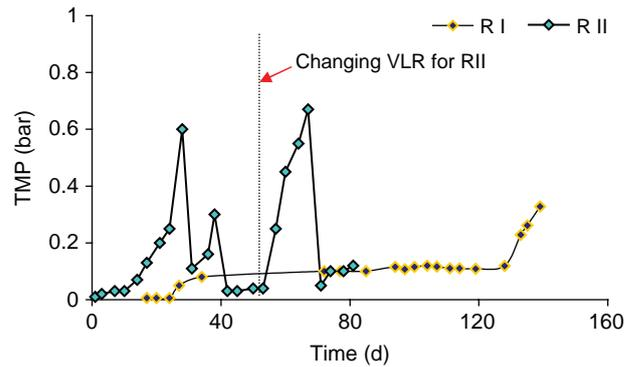
Fig. 2. TMP variation versus operating time during the MBRs operation.
