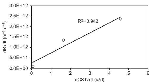
Fig. 3. Relationship between the CST and the second stage fouling rates of the MBR.
