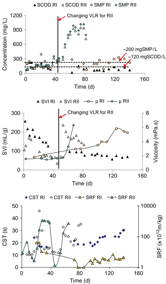
Fig. 1. The evolutions of physical sludge characteristics.
