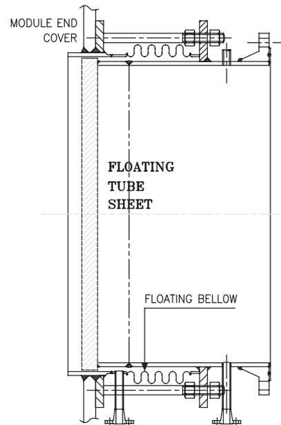
Fig. 5. Floating tubesheet joint.
