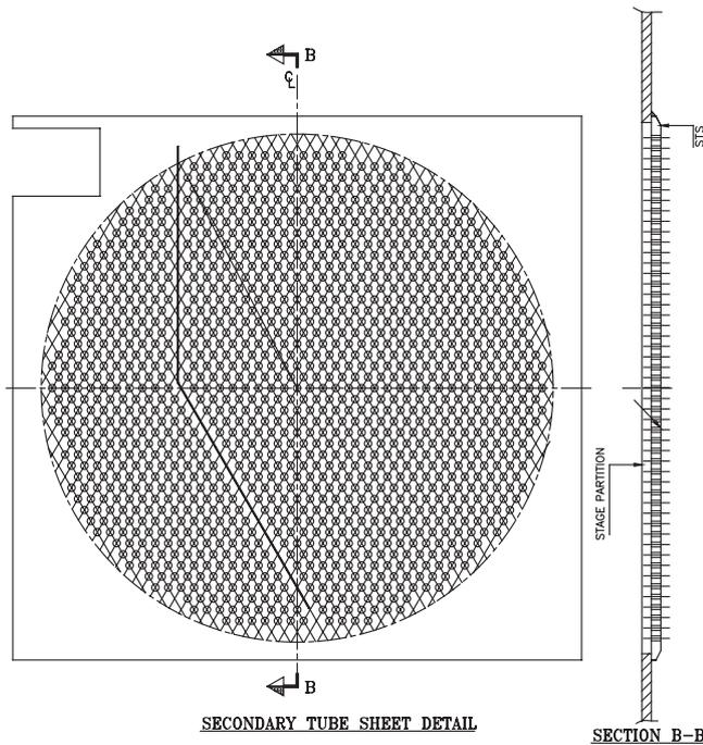
Fig. 10. Secondary tubesheet help reducing the leakage across stage partition.
