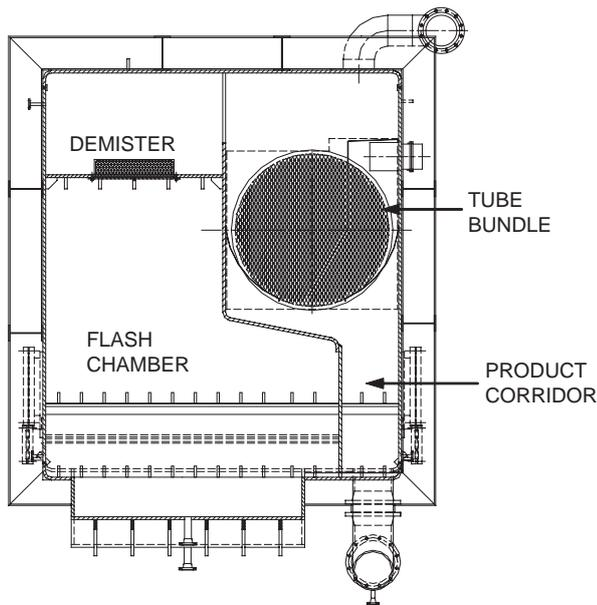
Fig. 4. Typical sectional view of MSF module.
