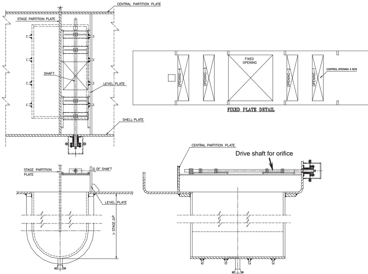
Fig. 9. Liquid seal and brine orifice.
