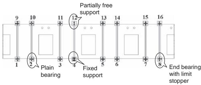
Fig. 7. Typical slide bearing mounting plan for module.
