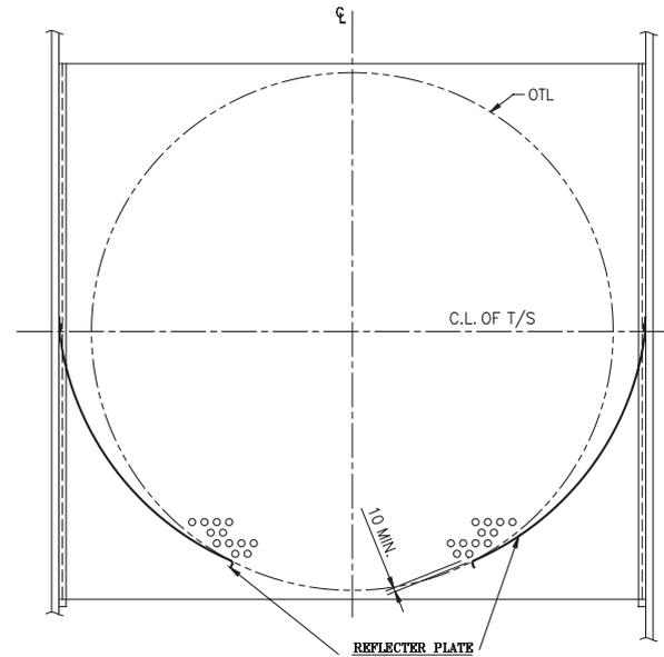
Fig. 11. Reflector plate increase resistance to vapor leakage to vent.
