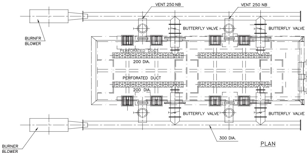
Fig. 12(a). Initial arrangement for stress relieving of mockup module.
