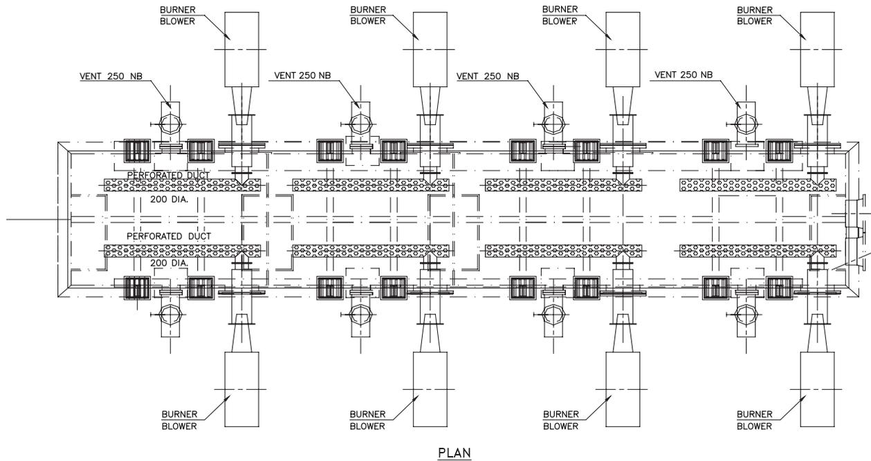
Fig. 12(b). Revised arrangements used for module stress relieving with individual burners for each chambers.
