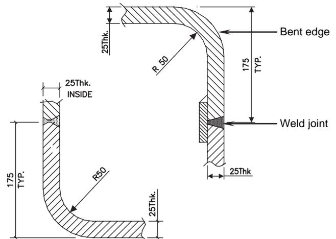
Fig. 3. Joints are shifted from the corners of the shell.
