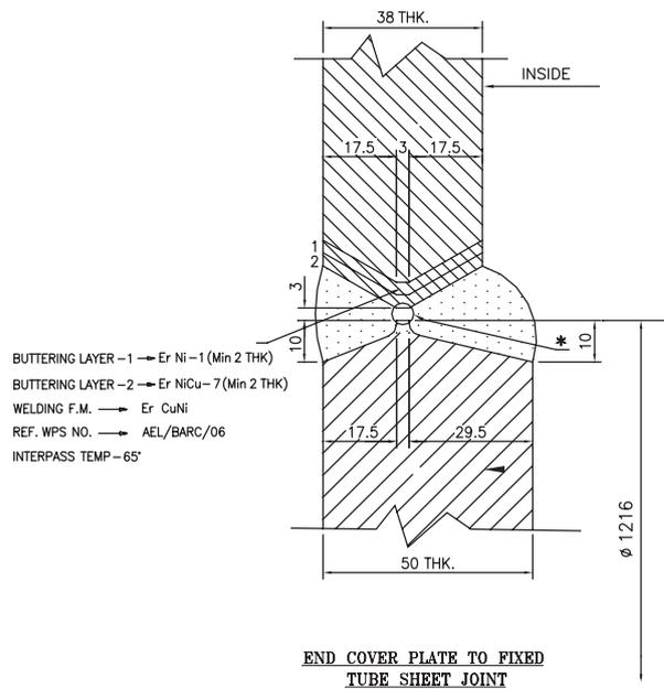
Fig. 13. End cover plate to fixed tube sheet joint.
