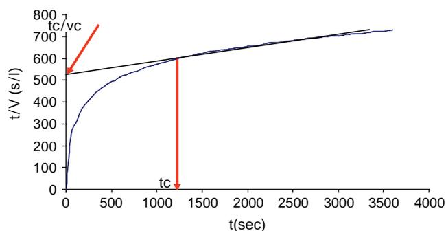
Fig. 2.  $t$  (time)/ $v$  (permeate volume) vs.  $t$  for feed water.
