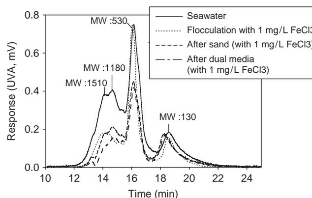
Fig. 3. MWD of SWOM (seawater organic matter) after different pretreatments.
