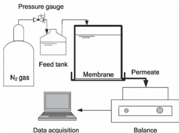
Fig. 1. MFI experimental setup.
