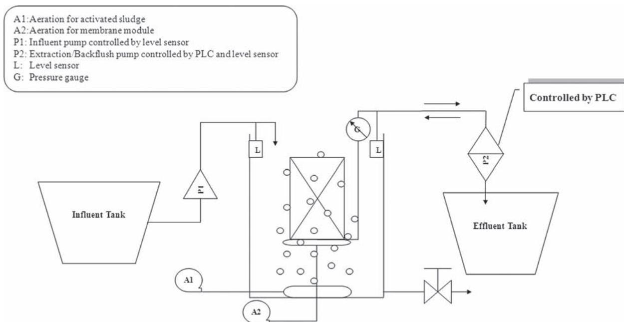
Fig. 1. Schematic diagram of MBR experimental setup.
