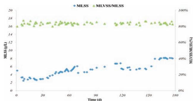
Fig. 3. Variation of MLSS concentration and MLVSS/MLSS ratio during this study.
