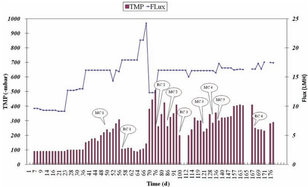
Fig. 4. Variations of membrane flux and TMP.
