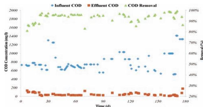
Fig. 2. COD removal in this MBR system.
