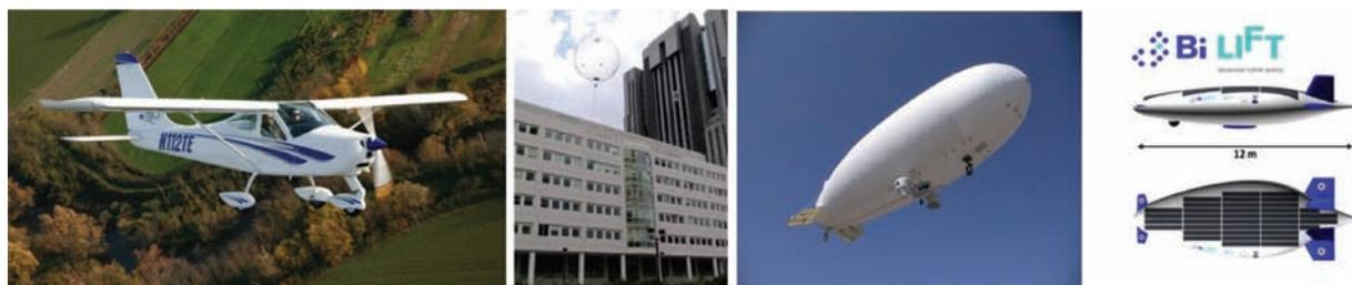
Fig. 2. ULM – Tethered Balloon – Blimp UAV – Hybrid LTA UAV.
