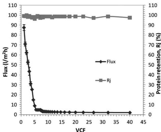
Fig. 3. Permeate flux and protein rejection versus VCF during ultrafiltration of fish mince wash water.
