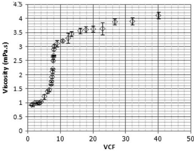
Fig. 4. Viscosity of retentate versus VCF during ultrafiltration of fish mince wash water.
