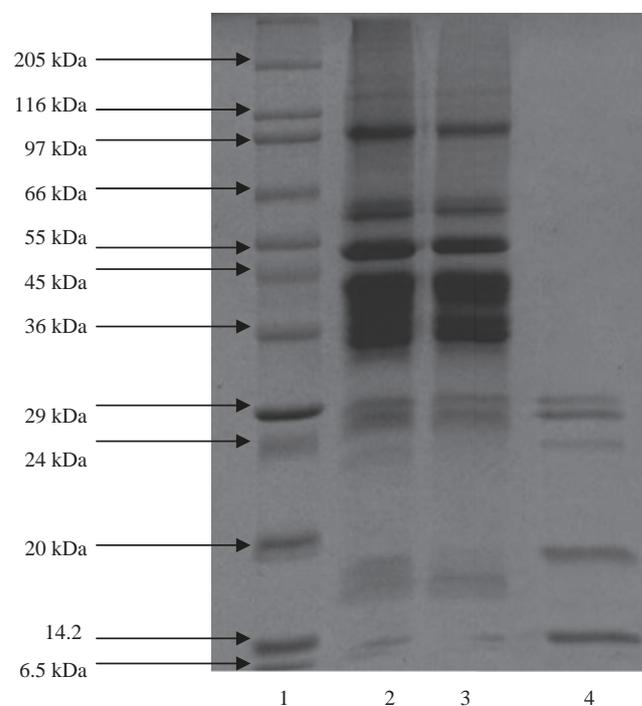
Fig. 1. SDS-PAGE pattern of fish mince wash water: (1) standard protein, (2) original, (3) concentrate (at VCF = 40) and (4) permeate.
