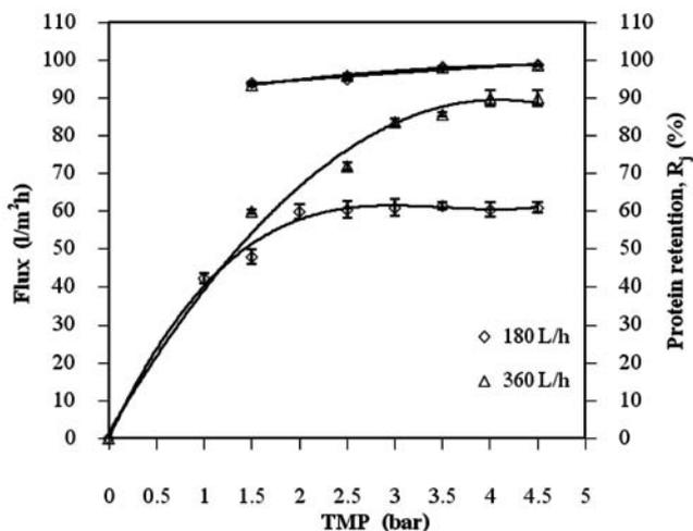
Fig. 2. Permeate flux and protein retention during ultrafiltration of fish mince wash water.
