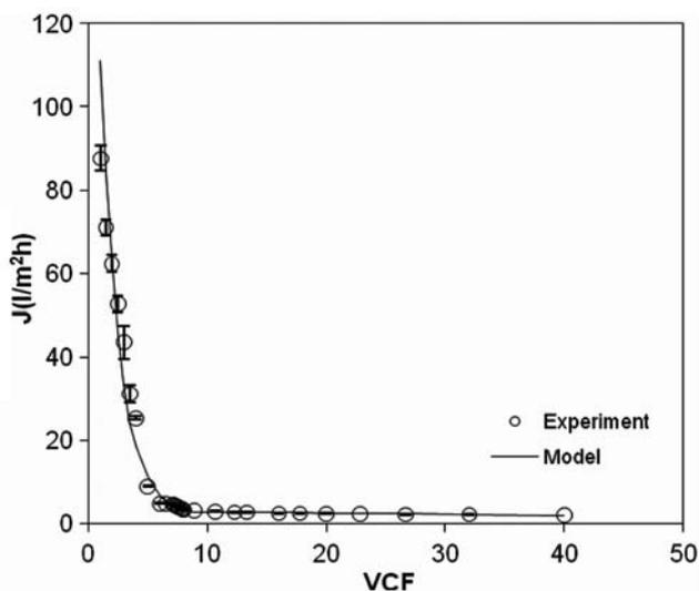
Fig. 6. Shear controlled model for fish mince wash water concentration by ultrafiltration.
