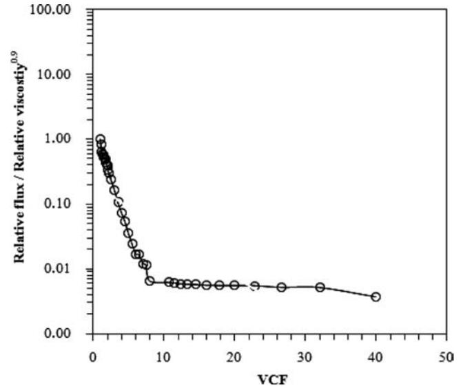
Fig. 5. Development of shear controlled model for ultrafiltration of fish mince wash water
