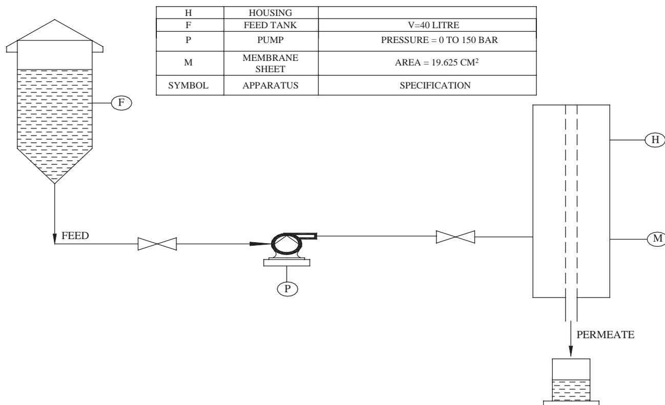
Fig. 2. Schematic diagram of the experimental apparatus setup.
