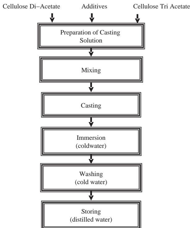
Fig. 1. Process block flow diagram for preparation of cellulose acetate membrane by casting.
