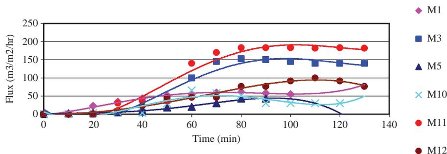
Fig. 4. Change of flux with time for different membranes.
