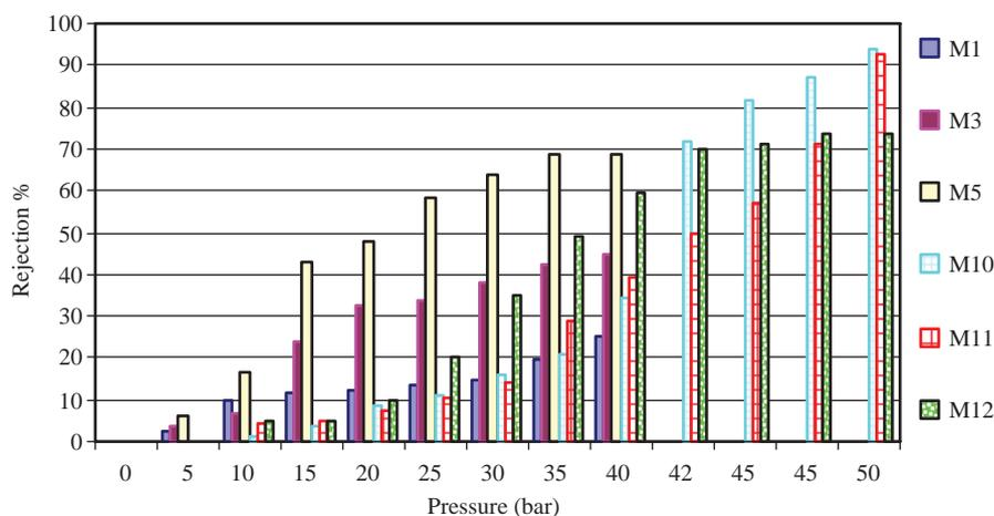
Fig. 7. Effect of applied pressure on water desalting efficiency for different membrane samples.
