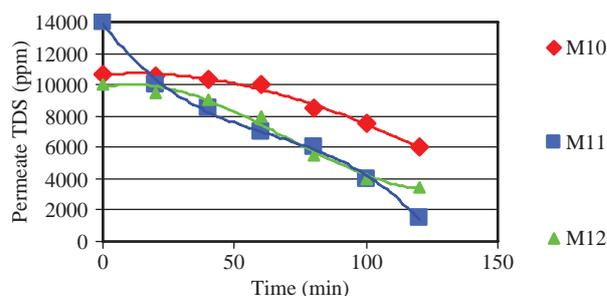
Fig. 6. Change of desalting efficiency with time at constant pressure (30 bar) for selected membrane samples.
