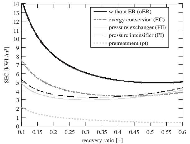
Fig. 7. Comparison of basic concepts – specific energy consumption versus recovery ratio for a seawater concentration of 35 g/l.
