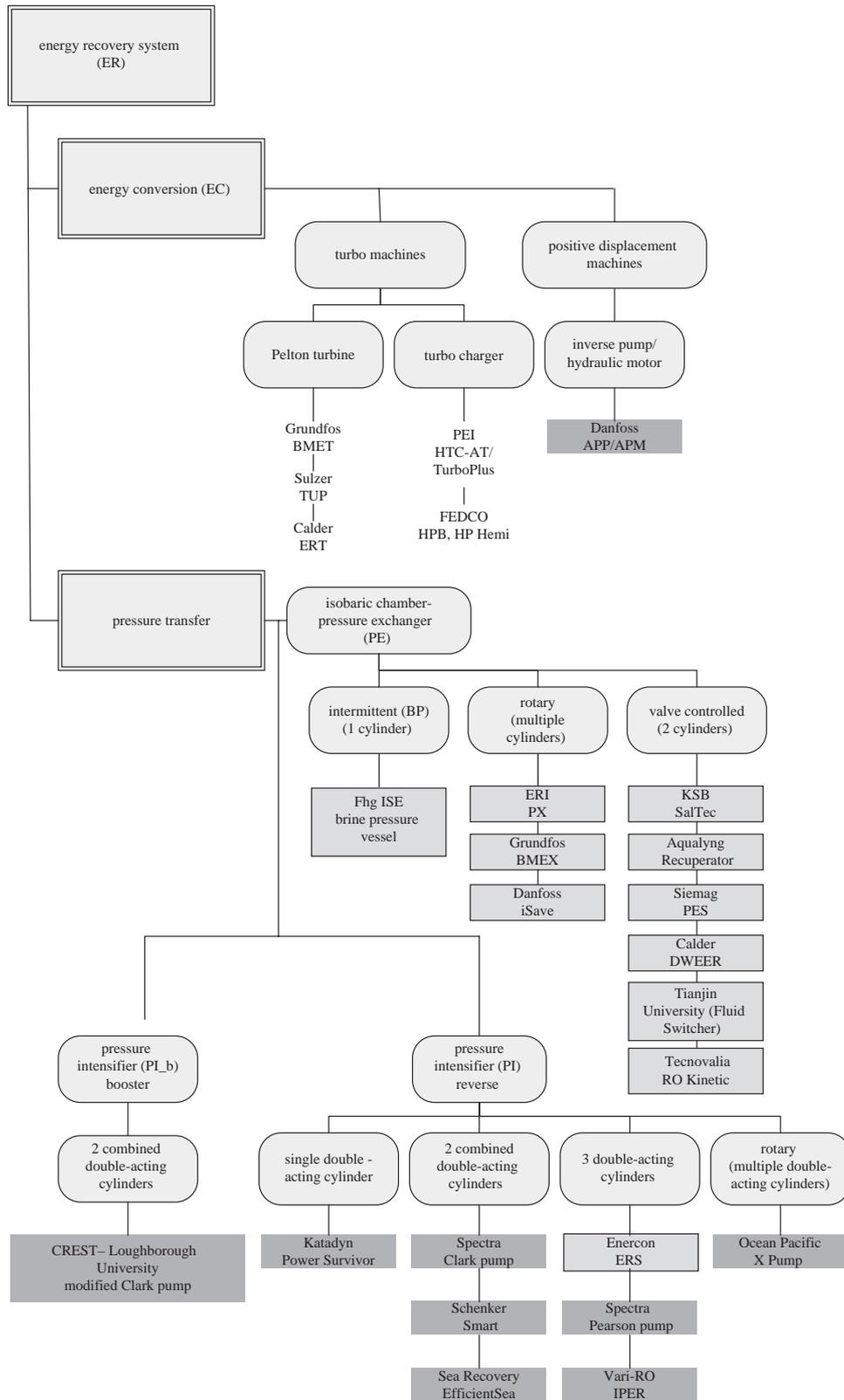
Fig. 6. Overview of energy recovery systems in the market sorted by their physical principle with examples of known products and companies; light hatching: suitable in principle; not available in the market or not available in the needed magnitude; dark hatching: suitable and available (this list is not exhaustive).
