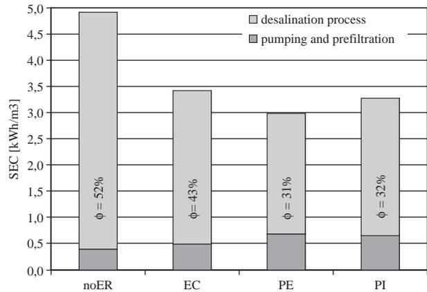
Fig. 8. Comparison of basic concepts – minimum of specific energy and corresponding best recovery ratios.
