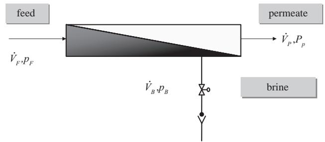
Fig. 1. RO concept without energy recovery (noER).
