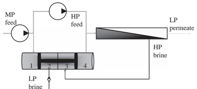
Fig. 5. RO concept with pressure intensifier (ER-PI).
