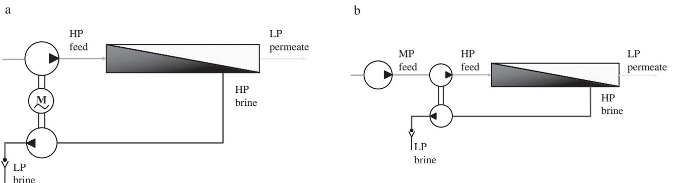
Fig. 2. (a) ER-EC with single shaft and (b) ER-EC with turbocharger and separated pump.
