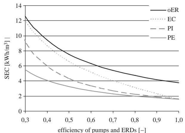
Fig. 9. Part load behaviour of RO concepts; specific energy consumption over the efficiency of pumps and energy recovery devices.
