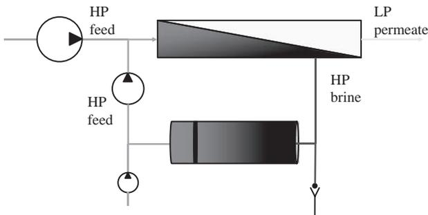
Fig. 4. RO concept with a brine pressure vessel for a batch process (ER-BP).
