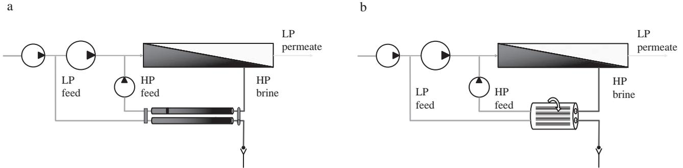
Fig. 3. (a) RO concept with a valve controlled pressure exchange unit (ER-PE). (b) RO concept with rotary pressure exchange unit (ER-PE).
