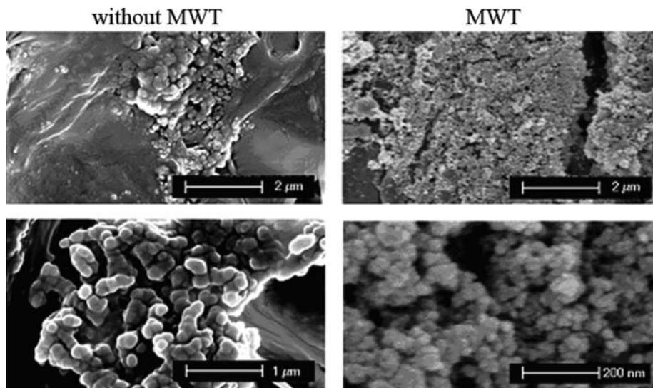
Fig. 5. The comparison of particles dispersed in outlet hot water.
