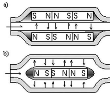
Fig. 1. Basic schemas of MWT devices: (a) perpendicular (parallel arrangement of permanent magnets), (b) radial (kernel of electromagnetic coils inserted into ferromagnetic tube).
