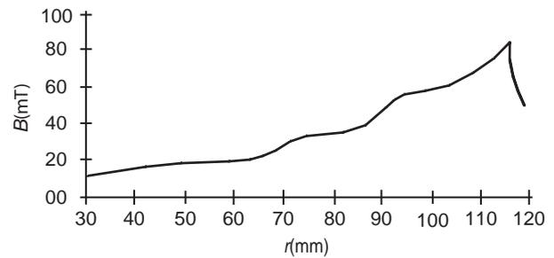
Fig. 7. The magnetic-field density distribution in the gap along the radius of inner plate in MWT device with flat coil.
