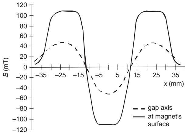
Fig. 2. The magnetic flux distribution in the rectangular gap between two rows of alternately arranged NiFe magnets (2 cm long and separated with 0.5 cm wide segments).
