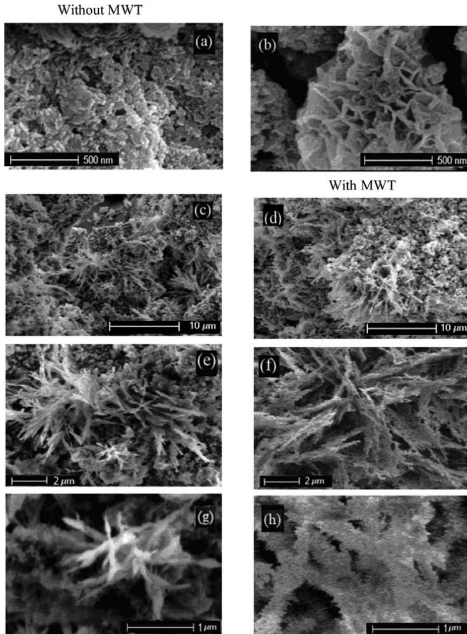
Fig. 8. Micrographs of the scale from the bottle-washing machine. (a–e) Sample from untreated water, (f–h) Sample from magnetically treated water.
