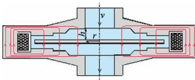
Fig. 6. MWT device with flat coil.
