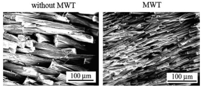
Fig. 3. Micrographs of scales on the heating spiral [28].
