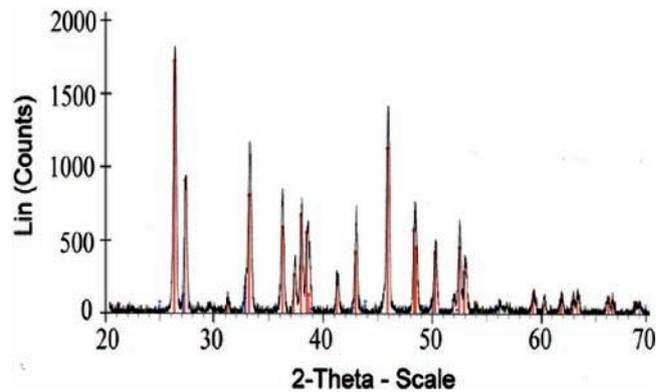
Fig. 4. X-ray diffraction spectrograph of particles dispersed in outlet hot water, identifying the sample as aragonite.
