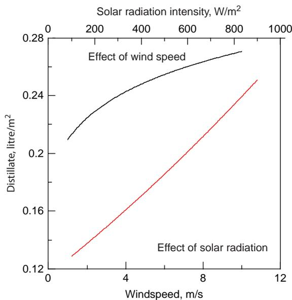
Fig. 11a. Effect of wind speed and solar radiation intensity on the solar still production.
