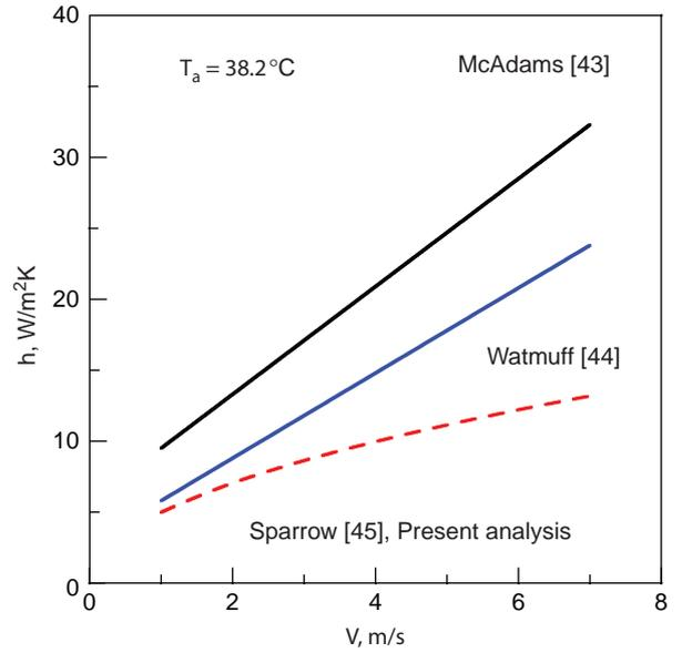
Fig. 2b. External convection heat transfer coefficient due to wind speed.
