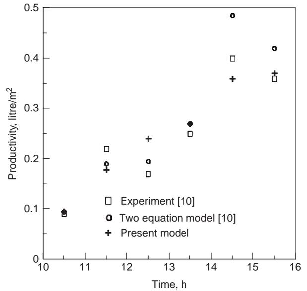
Fig. 3b. A comparison of the hourly still productivity with Nijmeh et al. [10].
