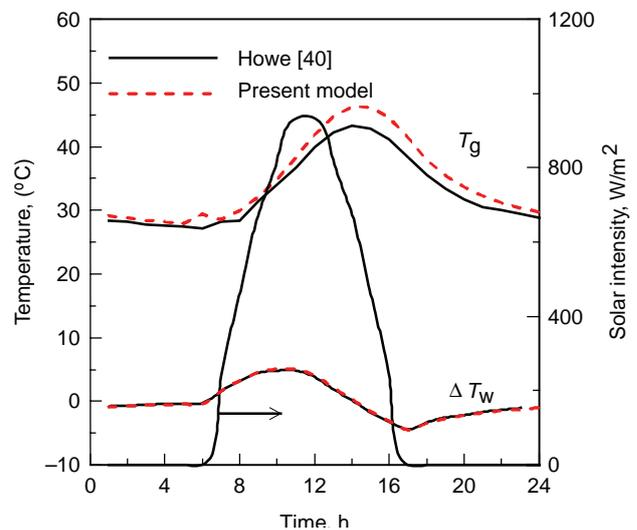
Fig. 5. Comparison of incremental basin water temperature change and glass temperature with time: comparison with Howe data [33].
