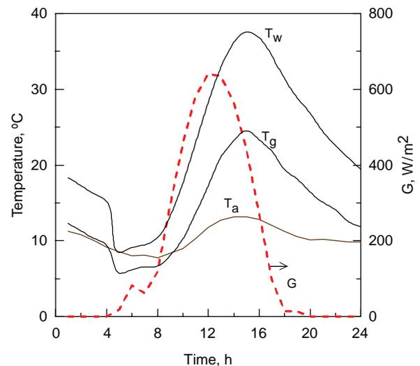
Fig. 9. Temperatures and solar radiation in a typical winter day in Dhahran.
