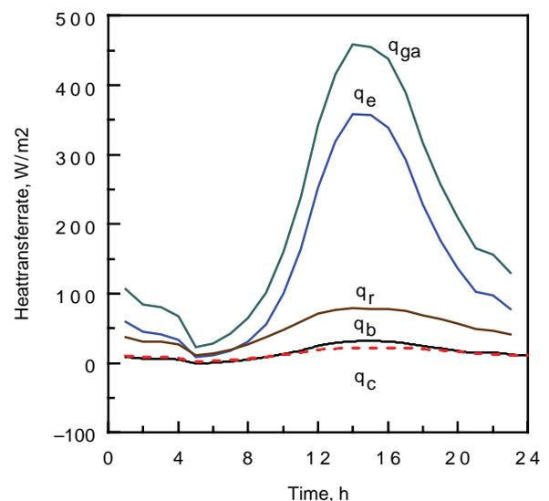
Fig. 6. Various components of heat transfer rate in a typical summer day in Dhahran.
