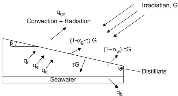
Fig. 1. Solar still geometry and energy transfer mechanisms.
