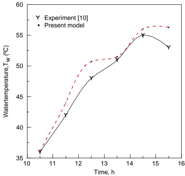
Fig. 4a. A comparison between calculated and measured [10] water temperature.
