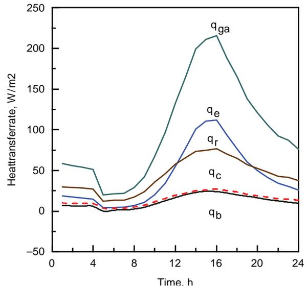
Fig. 8. Various components of heat transfer rate in a typical winter day in Dhahran.
