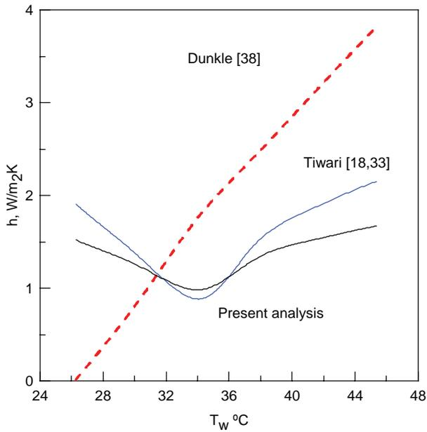
Fig. 2a. Convection heat transfer coefficient within the still.
