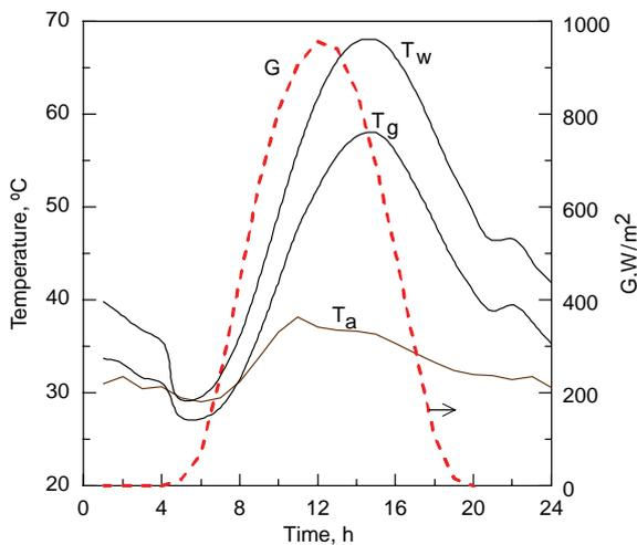
Fig. 7. Temperatures and solar radiation in a typical summer day in Dhahran.
