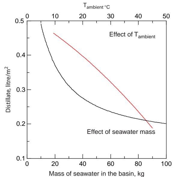
Fig. 11b. Effect of mass of seawater in the basin and ambient temperature on solar still production.
