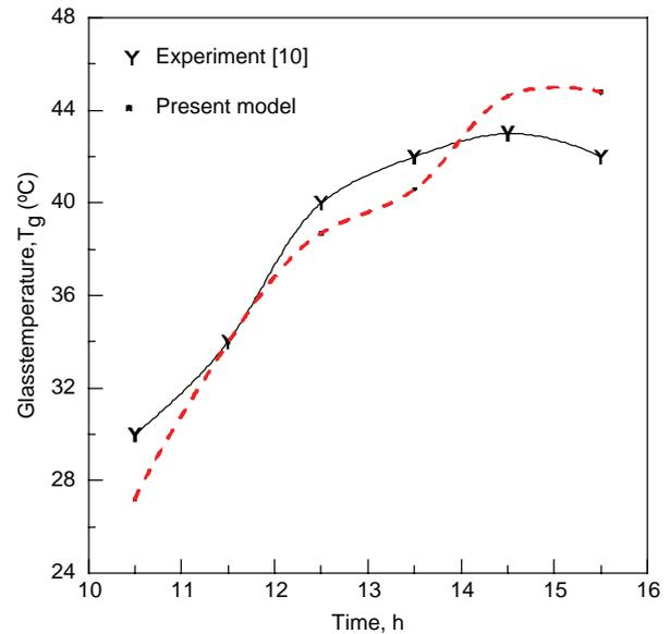
Fig. 4b. Fig. 3a: A comparison between calculated and measured [10] glass temperature.
