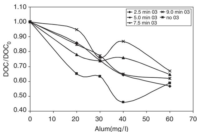
Fig. 3. The effect of pre-ozonation on DOC removal by alum coagulation.
