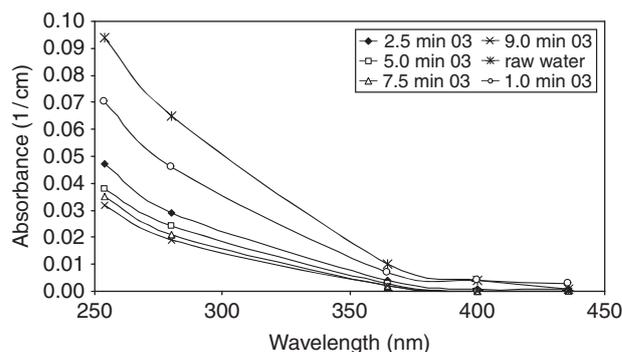
Fig. 2. Effect of ozonation time periods on the absorbance removal at different wavelengths.
