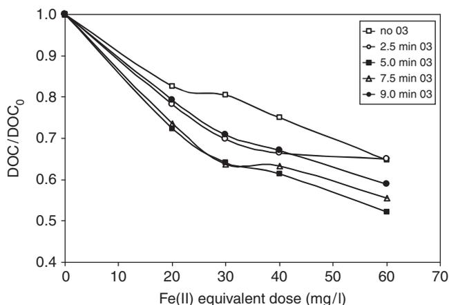
Fig. 4. The effect of pre-ozonation on DOC removal by ferric chloride.
