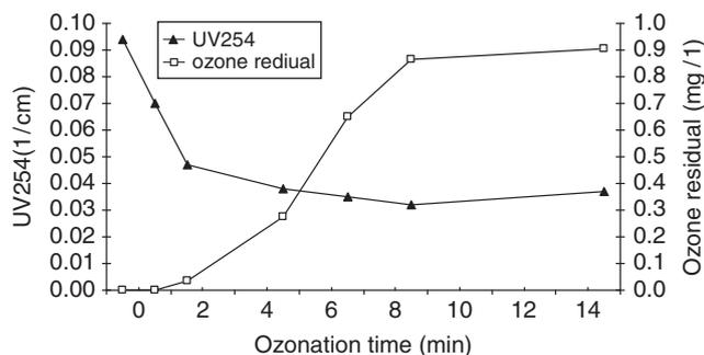
Fig. 1. Ozone demand and  $\text{UV}_{254}$  removal with respect to ozone contact time.
